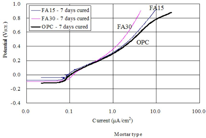
Figure 6. Anodic Polarization Curves of Mortars without Chloride
