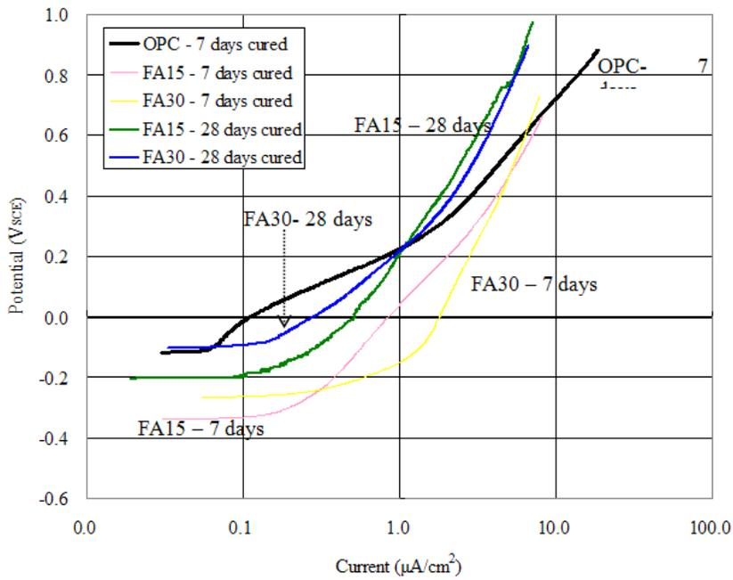
Figure 7. Anodic Polarization Curves of Cl-contaminated Mortars
