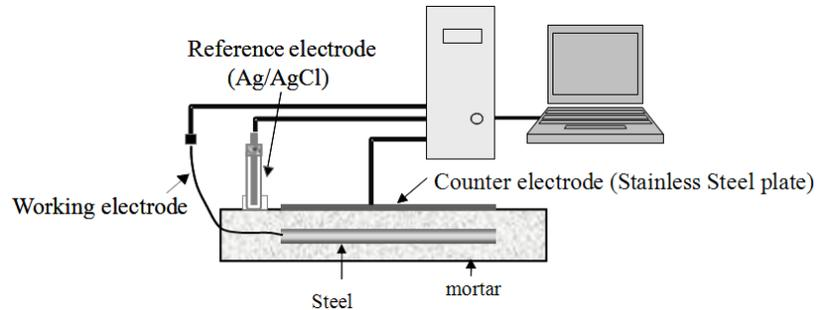
Figure 3. Setup for Anodic Polarization Test
