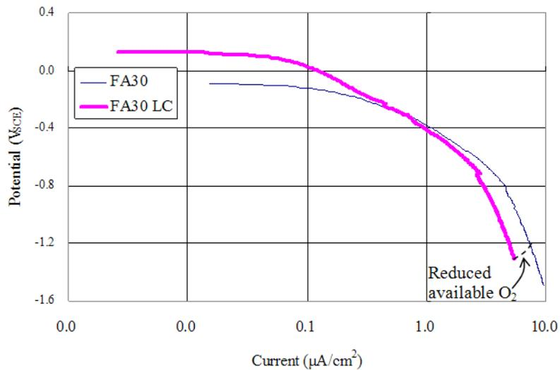
Figure 9. Cathodic Polarization Curves for FA30
