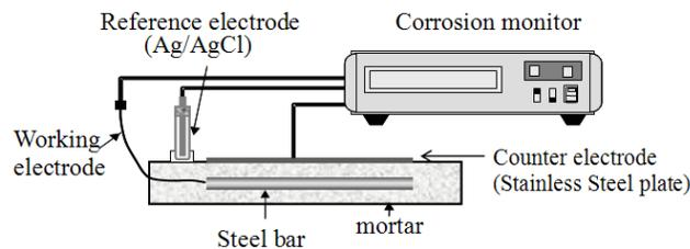
Figure 2. Measurement Setup for Corrosion Potential and Current Density
