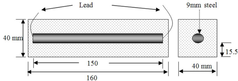
Figure 1. Detail of the Reinforced Mortar Specimen
