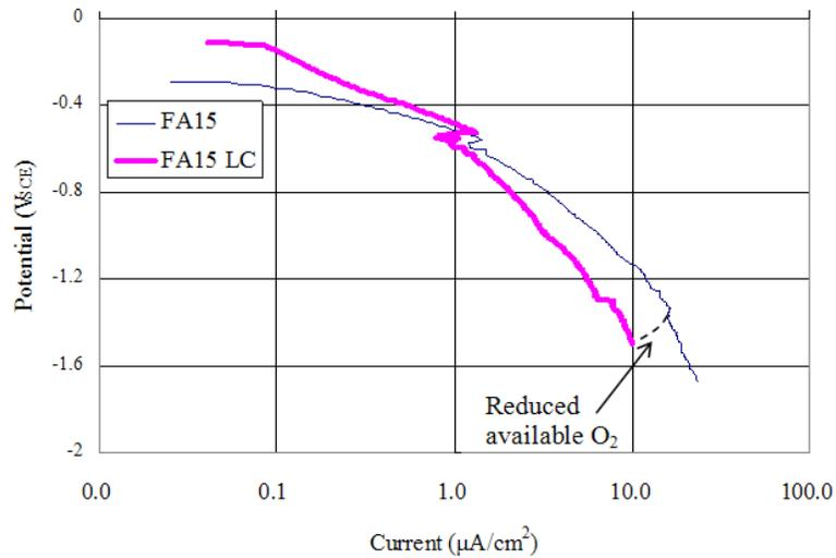
Figure 8. Cathodic Polarization Curves for FA15
