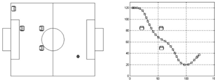
Figure 17. Test Case 12 and Sample Robot and Ball Trajectories Using the Bezier Curvature Algorithm
