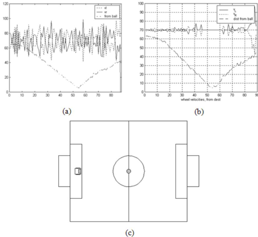
Figure 18. Variation of wheel velocities when using the (a) uni-vector algorithm and (b) bezier curvature algorithm for test case 1. (c) Robot and ball placement for test case 1.
