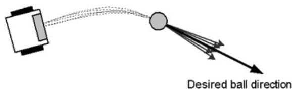
Figure 14. The noise added by the simulator causes the robot to traverse different paths during each execution.
