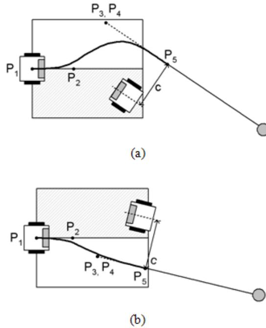
Figure 7. (a) Control points when the obstacle is to the right of the robot. (b) Control points when the obstacle is to the left of the robot.
