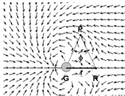
Figure 10. Computation of the Direction of the Uni-Vector Field
