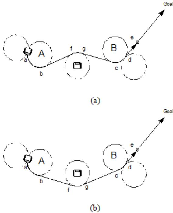
Figure 12. Paths Generated by the Line-Circle Algorithm with an Obstacle Present
