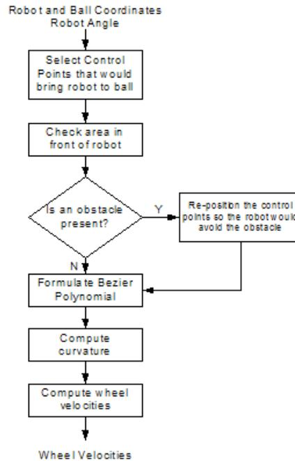
Figure 4. Computation of Wheel Velocities Using the Bezier Curvature Algorithm
