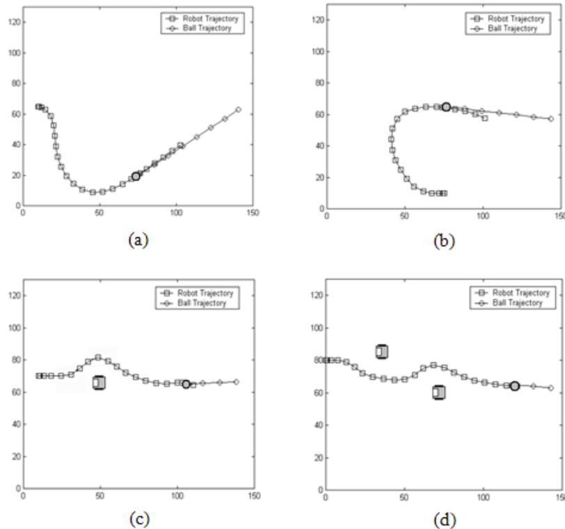
Figure 15. Robot and Ball Trajectories Using the Bezier Curvature Algorithm
