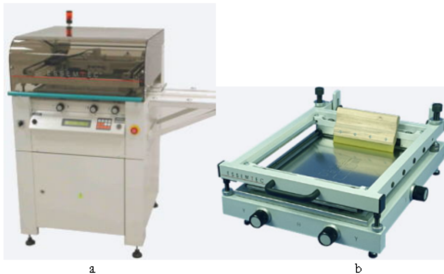
Figure 1. Screenprinting equipment a) Automatic printer was used for low speed (10 mm/s up to 100mm/s printing b) table top printer was used for high speed printing (more than 100 mm/s)
