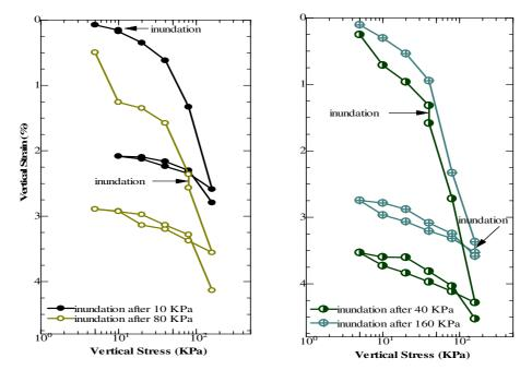
Figure 5 Stressvs strain plot indicating strain due to inundation of wastes from aggregate quarry from Cavite (TS#1)
