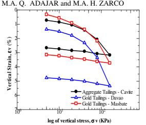
Figure 3. Stress-strain curve of tailings from oedometer test
