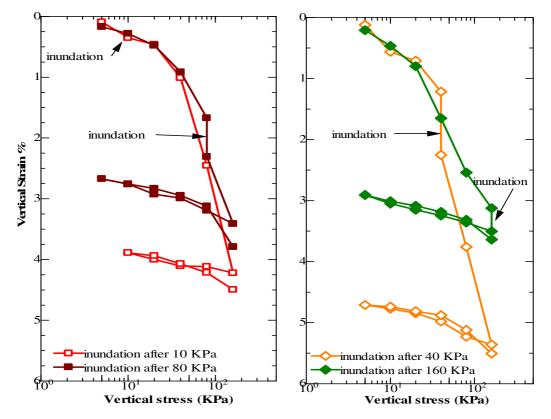
Figure 7 Stress vs. strain plot indicating strain due to inundation of gold mine tailings from Masbate (TS#3)
