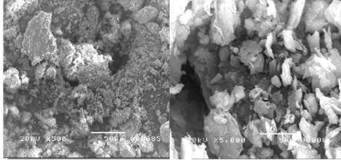
500X magnification 5000X magnification (c) Gold mine tailings from Masbate (TS#3)
