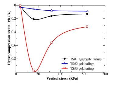
Figure 9 Plot of hydrocompression strain for each vertical stress
