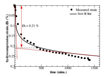
Figure 8 Typical test result in strain vs time plot used to measure hydrocompression strain
