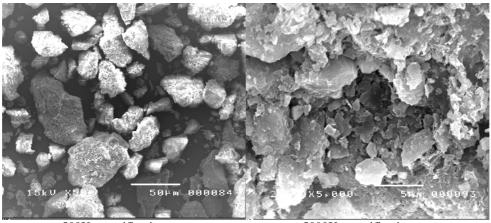
500X magnification 5000X magnification (a) Wastes from concrete aggregate quarry in Cavite (TS#1)
