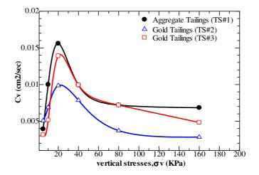
Figure 4. Time rate of consolidation of tailings against vertical stress
