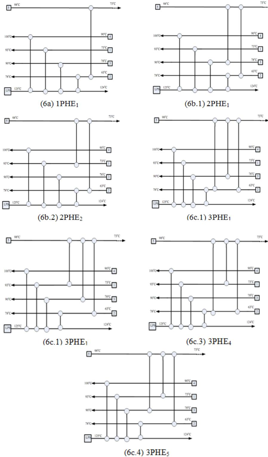
Figure 6. Feasible HEN above pinch for (6a) 1 PHE, (6b) 2PHE<sup>1</sup> and (6c) 3PHE<sup>1</sup>
