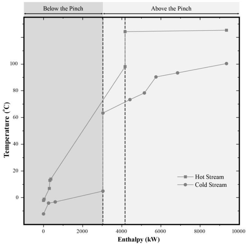
Figure 4d. Balanced composite curves
