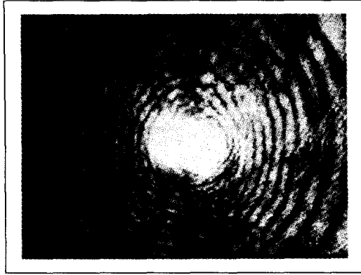
Fig. 4. Diffraction rings formed due to phase retardation of laser
