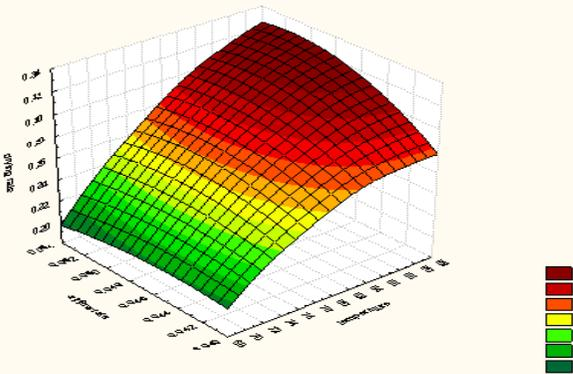
Figure 7a. Surface plot for drying rate vs. airflow rate and drying air temperature
