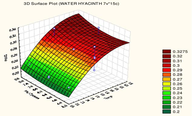
Figure 7b. Surface plot of drying rates as affected by drying air temperature and no. of passes through the roller
