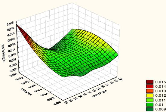
Figure 8a. Surface plot for tensile strength vs. airflow rate and drying air temperature
