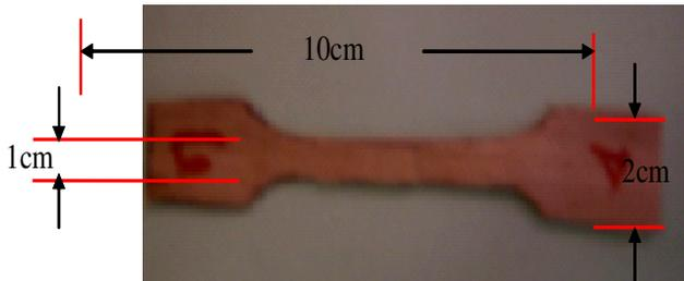
Figure 3. The tensile specimen
