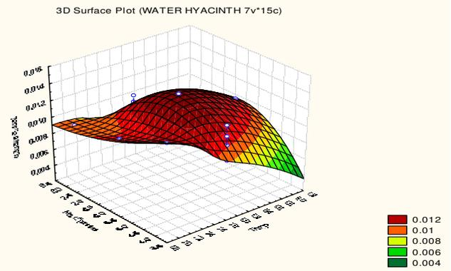
Figure 8b. Surface plot of tensile strength as affected by drying air temperature and no. of passes through the roller
