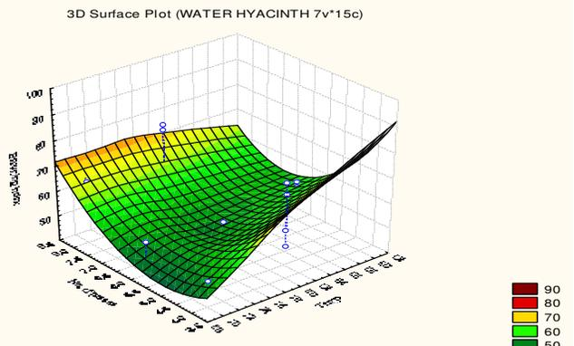
Figure 9b. Surface plot of browning index as affected by drying air temperature and no. of passes the roller
