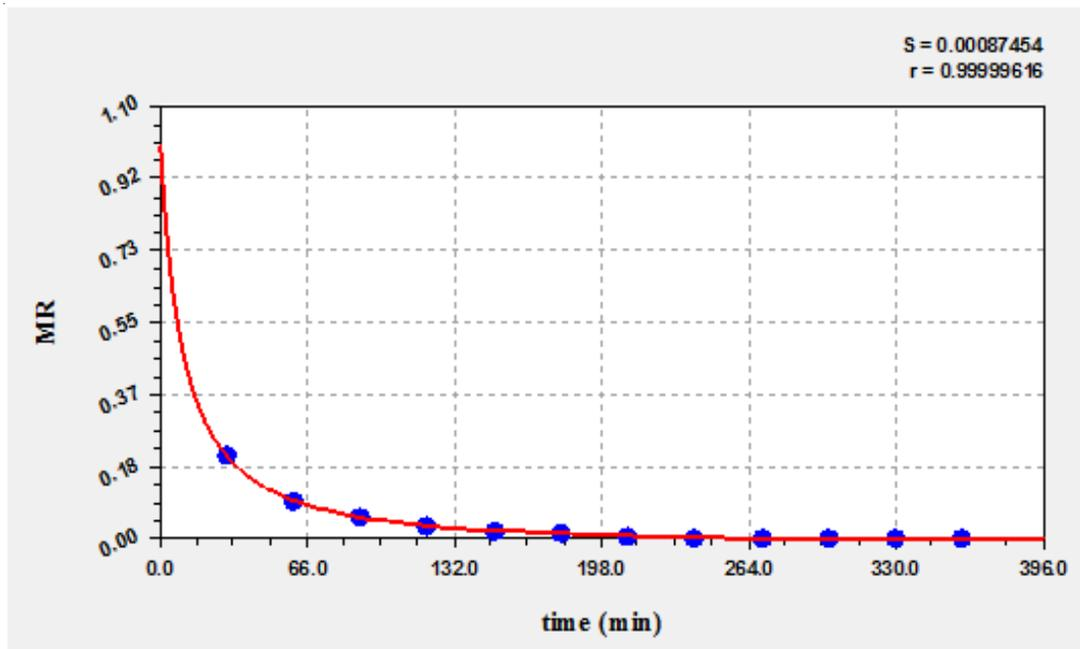
Figure 11. Moisture ratio vs. time of Run no. 6
