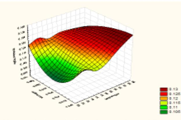
**Figure 6. Surface plot for moisture ratio vs. airflow rate and drying air temperature**
