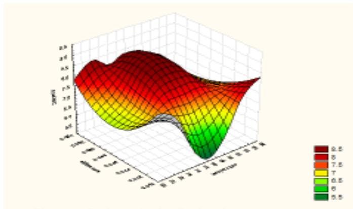
**Figure 5. Surface plot for final moisture content vs. airflow rate and drying air temperature**
