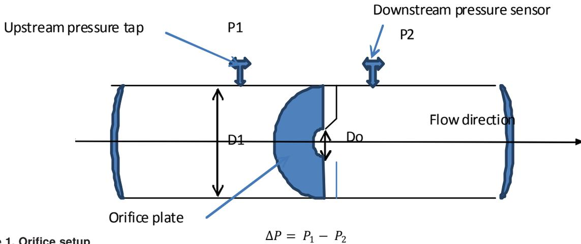
Figure 1. Orifice setup
