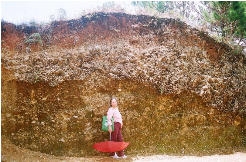
Figure 2: Example of a road cut at Mount Salat, Sitio Sagapa, Brgy. Palaypay, Kapangan, Benguet. Notice thin topsoil interspersed with 20-30cm Layer A zone, 20-50cm Layer B regolith. 600cm± Layer C is mother rock (Photo taken in 2008)
