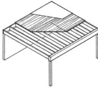
**Figure 24:** An illustration of a floor framing system consisting of floor joists and floor boards (Source: Building Construction Illustrated, 4<sup>th</sup> edition. This material is reproduced with permission of John Wiley and Sons, Inc.).
