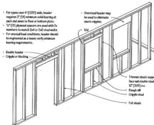
**Figure 23:** An illustration of what a stud wall looks like (Source: Building Construction Illustrated, 4<sup>th</sup> edition. This material is reproduced with permission of John Wiley and Sons, Inc.).
