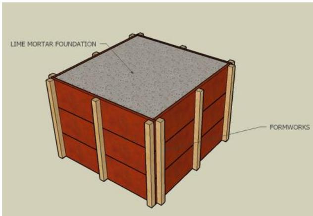
**Figure 13:** 3d rendition of how a column foundation is created (Illustration by Angelus Sales).
