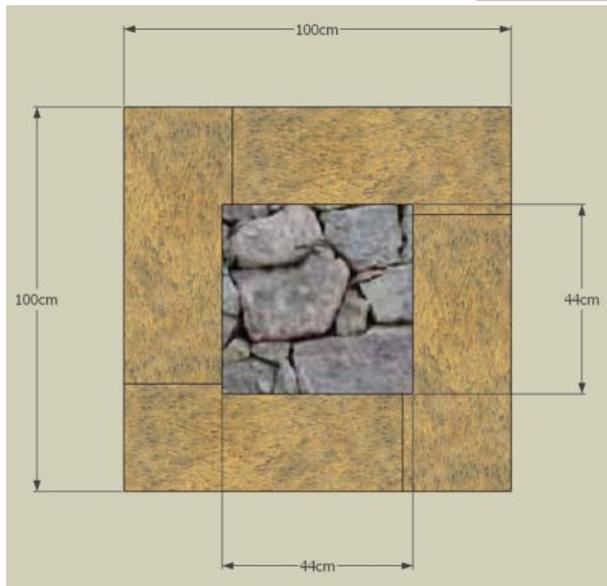
**Figure 18:** Plan view of the stone columns enclosed by adobe blocks (Illustration by Angelus Sales).
