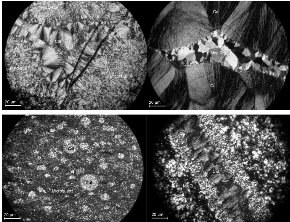
**Figure 5.** Micrographs of the observed minerals in the thin sections, where Cal is chalcedony *s.l.*, Meq Q is mega-quartz, and Mic Q is micro-quartz
