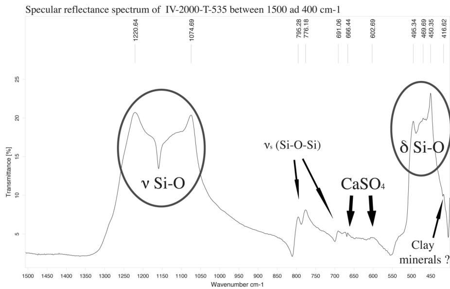
**Figure 4.** IR spectrum of a flake showing the characteristic absorptions
