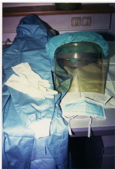
Figure 3a (above) and b (left). In order to guarantee further analyses under sterile conditions, special working areas (e.g. clean bench) and clothes (e.g. latex gloves and plexiglass face masks) have to be used in sample processing.
