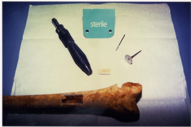
Figure 5 (left). Specific milling and separation tools used for the removal of contaminants possibly attached to the surface of a sample.
