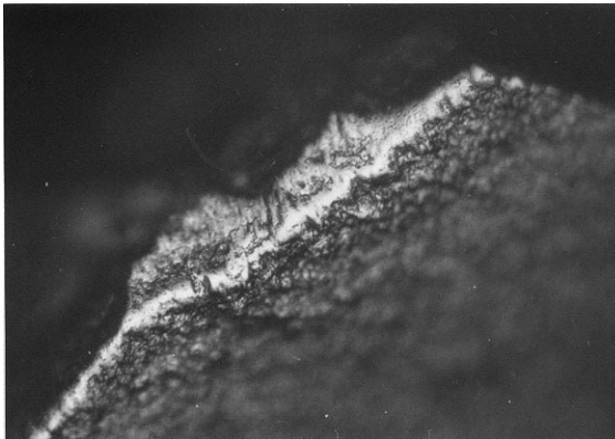
Plate 4 Polish bevel on tool edge caused by working on ivory (scale 320:1).
