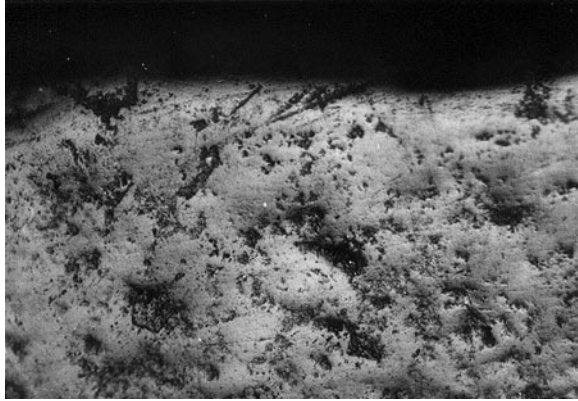
Plate 5 Micropitting on plant polish (scale 150:1).
