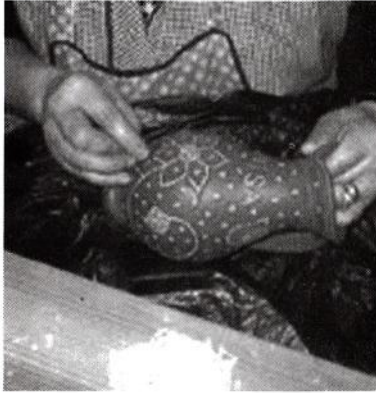
Inlaying of bits of quartz on the pottery performed by women. Each piece is inlaid one by one from a bunch of quartz bits on a small pile on the table.
