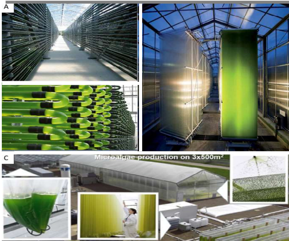
Figure 2. A closed-system type of photobioreactors. A. Tubular photobioreactor in Klötze, Germany Photo ® Jörg Ullmann (Masojidek & Torzillo, 2008), B. Flat-plate photobioreactor known as "Hanging Gardens" developed by ecoduna-produktions GmbH in Bruck/Leitha, Austria Photo ® ecoduna (Mohr, 2013), and C. Foil photobioreactor set-up by the NOVAgreen company in Bergheim-Neideraussem, Germany (Schreiber et al., 2017).
