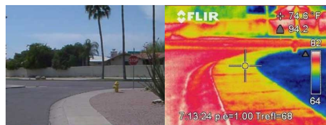
Figure 2: Actual and Infrared image showing high heat absorbing (low albedo) materials versus low heat absorbing (high albedo) materials. Blue colored region at the right is a gravel paved area. From: http://www.invisiblestructures.com/GreenBuilding1/heatisland.htm
