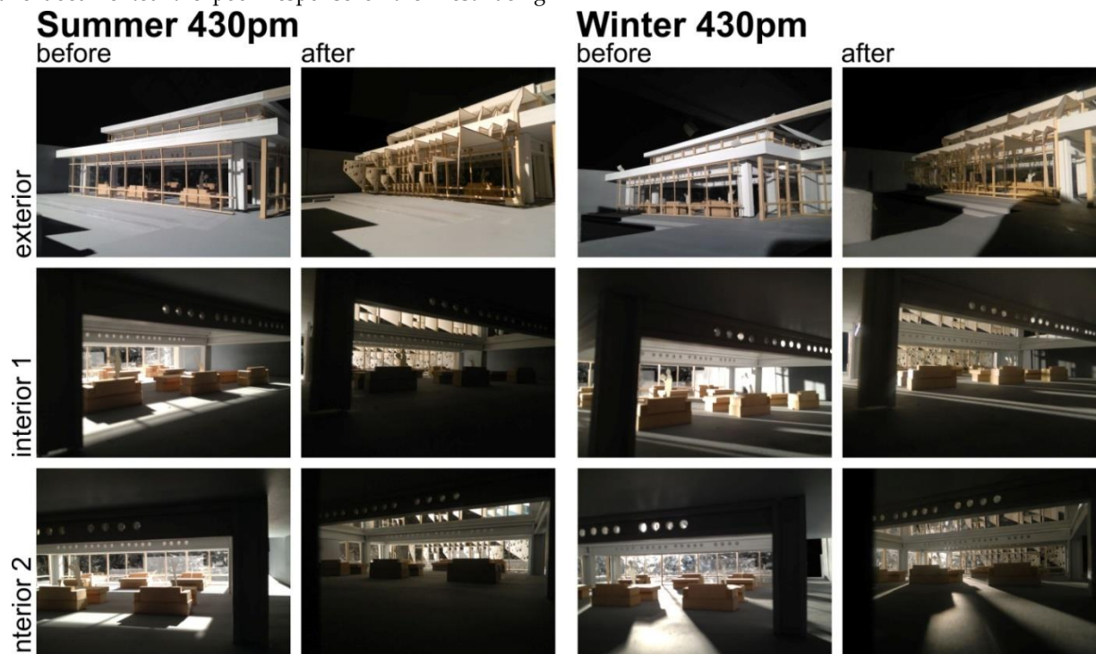
Figure 7. This matrix shows "before and after" photographs of the shading design (by B. Moges and C. Ayers), simulated at 430 pm, solar time, during the summer solstice, Jun 21, and the winter solstice, Dec 21. Note solar exclusion in summer and solar access in winter. The top row shows an exterior view; the next two rows display two interior views.
