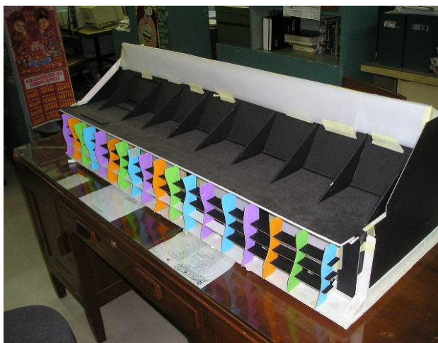
Figure 4. Daylight Model exterior.
