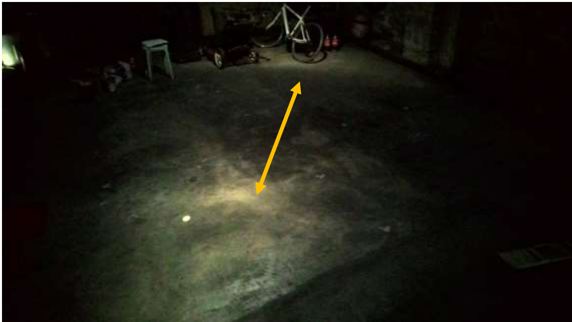
Figure 16. Light spread on the floor with floor distinct shadows in the middle, or in between the lit areas.
