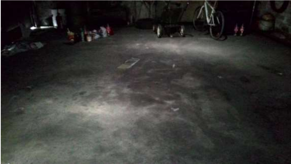
Figure 15. Light spread on the floor with two distinct areas of relatively high illuminance.
