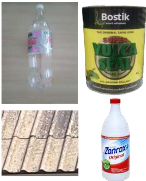
Figure 1 (clockwise from top left). 1.5L plastic bottle to be filled with filtered water; Epoxy /rubber sealant; Bleach; and Galvanized Iron sheet to match existing roofing.
