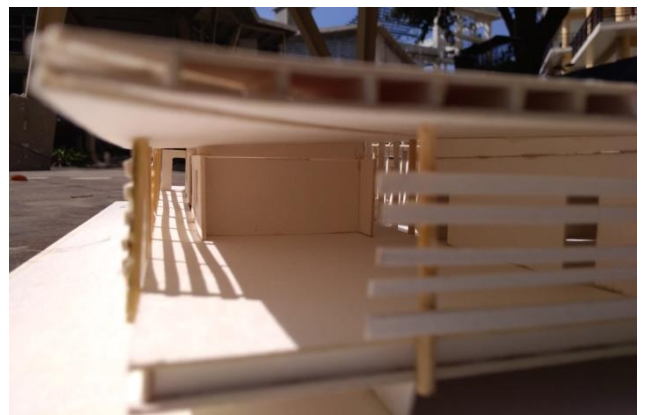
Figure 17. Eave and sunshade detail simulating Dec 21, 4pm. Source: Project and photo c/o Marc Carbon ad Rafael Sta. Maria (submitted student work)
