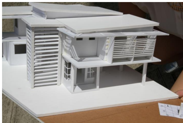
Figure 12. Testing the effectiveness of the horizontal sunshade devices of a monochromatic model. Source: Project and photos c/o Gilbert Bercero and Carina Morente (submitted student work)
