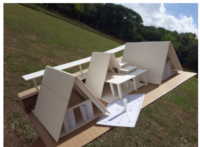
Figure 10. Student simulating the lightweight model under the sun with a steep angle rotation. Source: Project and photo c/o Ysabelle Coelyn Bacila (submitted student work)
