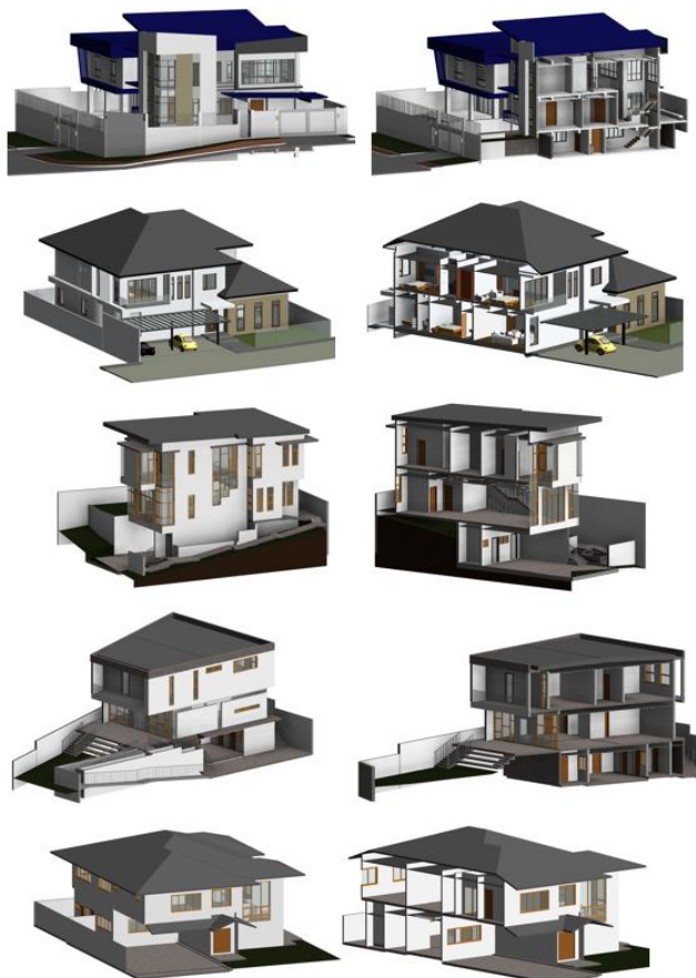
Figure 8. 3D Revit BIM models of Actual Projects.
