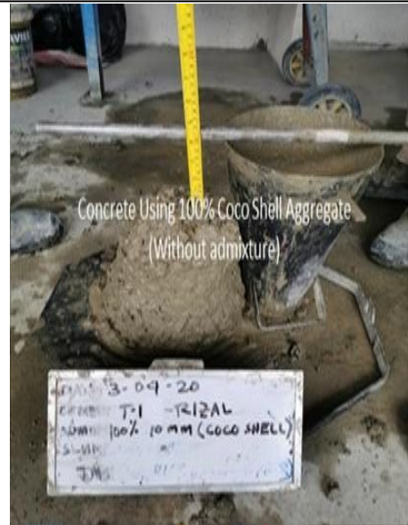
Figure 12. 100% Coconut Shell (0% Admix)
