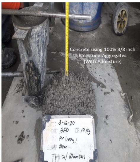
Figure 11. 0% Coconut Shell (1% Admix)
