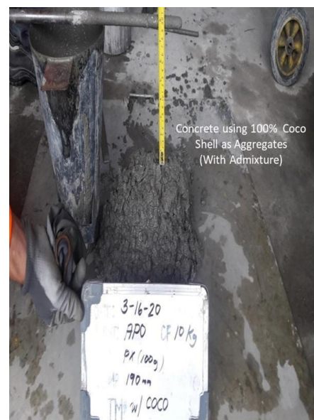
Figure 13. 100% Coconut Shell (1% Admix)
