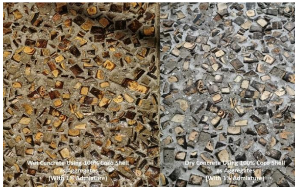
Figure 15. Wet and Dry Concrete with 100% Coconut Shell (1% Admix)
