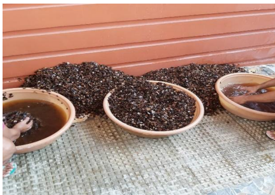
Figure 7. Washing of Soaked Sample
