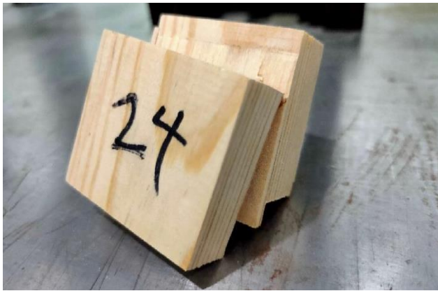
Figure 5. Aftermath of Shear and Delamination Test in Accordance with ASTM D905 (1998).
