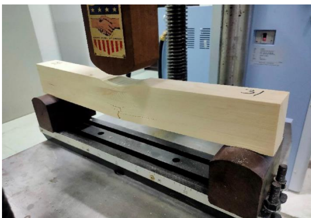
Figure 6. Aftermath of Static Bending Test in Accordance with ASTM D198 (2015).
