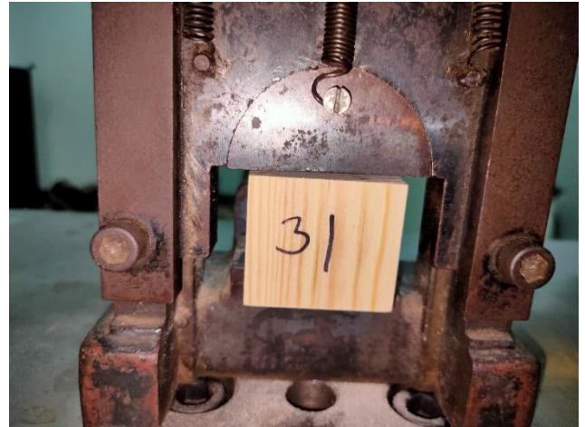
Figures 3. Shear test procedure in accordance with ASTM D905 (1998).
