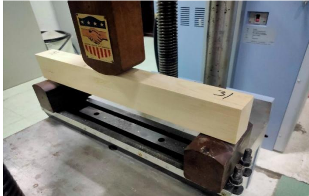
Figures 4. Flexure test procedure in accordance with ASTM D198 (2015).
