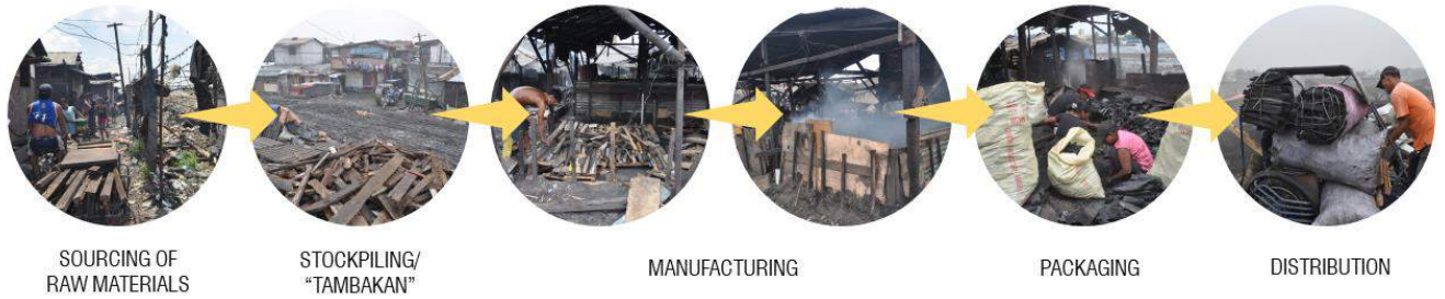
Figure 4. Charcoal production process. Source: Olivia Alma G. Sicam, 2013.
