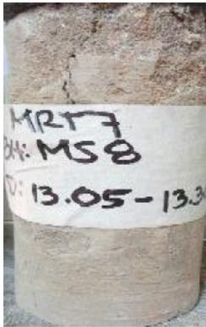
Figure 4. Rock core sample failed in shear
