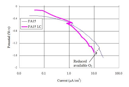
Figure 8. Cathodic Polarization Curves for FA15
