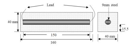
Figure 1. Detail of the Reinforced Mortar Specimen
