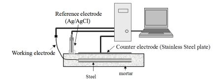
Figure 3. Setup for Anodic Polarization Test
