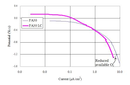
Figure 9. Cathodic Polarization Curves for FA30
