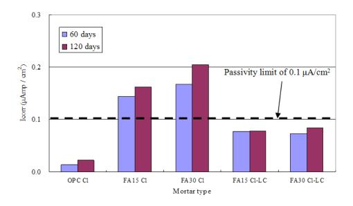
Figure 5. Corrosion Current Density
