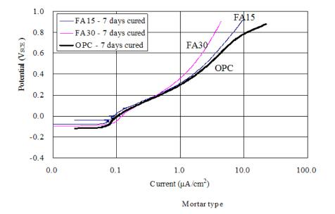
Figure 6. Anodic Polarization Curves of Mortars without Chloride
