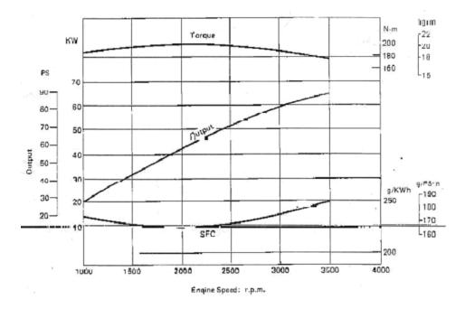
Figure 1. Engine Performance Curves from Manufacturer.
