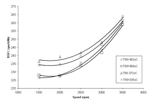
Figure 4. Graph of Brake Specific Fuel Consumption vs. Engine Speed.
