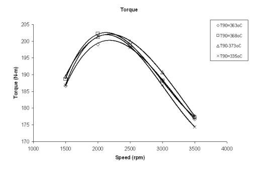
Figure 2. Graph of Brake Torque vs. Engine Speed.
