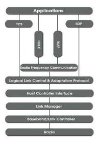
Figure 1. The Bluetooth Protocol Stack
