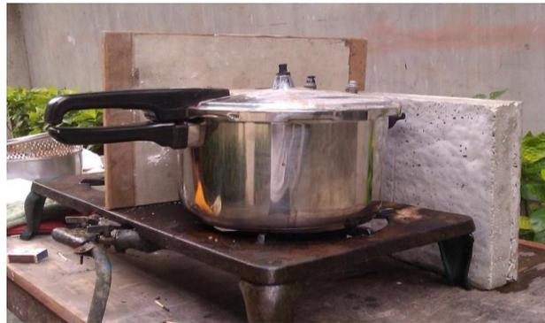
**Photo 2:** Shells Deproteinized in Pressure Vessel for 6 hours
