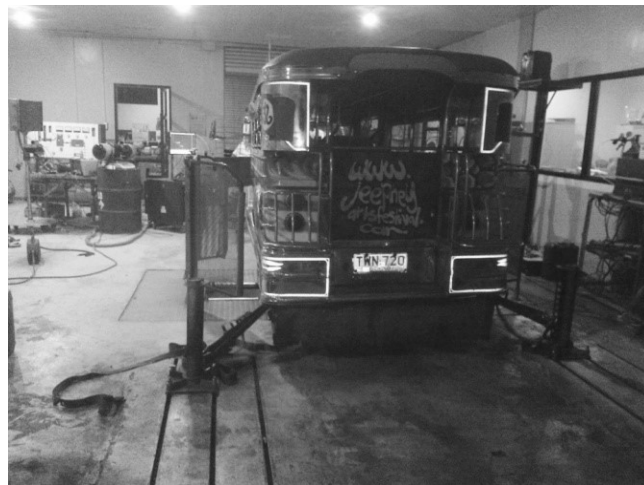
Figure 5. Test jeepney on chassis dynamometer, rear view
