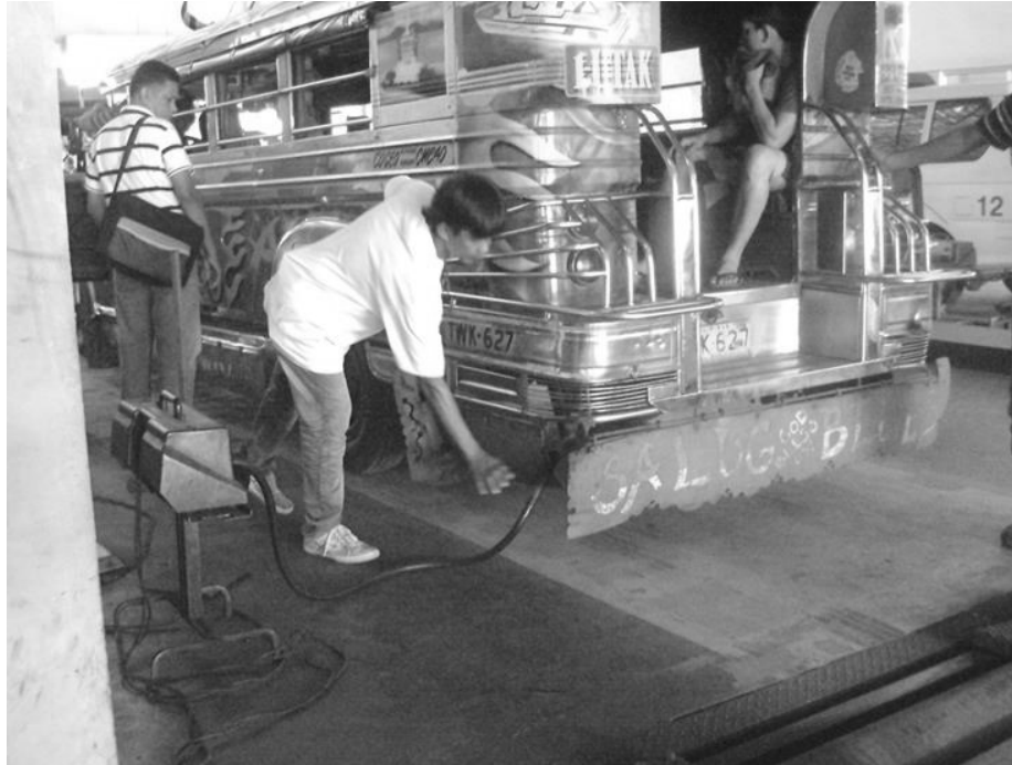
Figure 1. Jeepney unit during MVIC “pass/fail” smoke opacity tests
