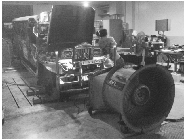
Figure 4. Test jeepney on chassis dynamometer, front view
