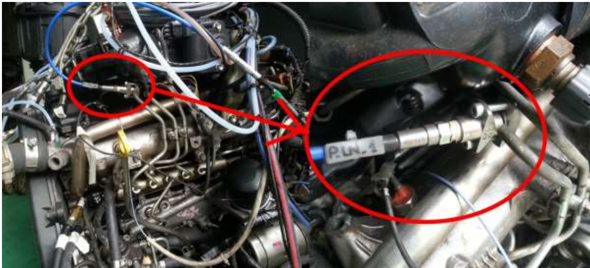
Figure 3: Toyota 1KD-FTV Engine, showing exact location of Line Pressure Sensor
