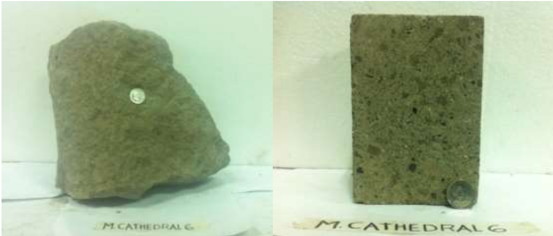
Figure 2. Images before and after cutting of the MC 6 specimen
