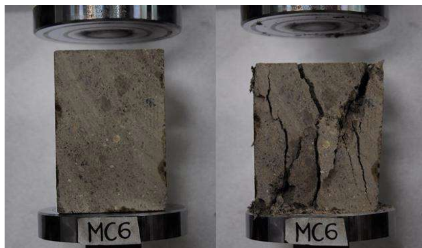
Figure 5. Specimen MC 6 before and after going through destructive testing
