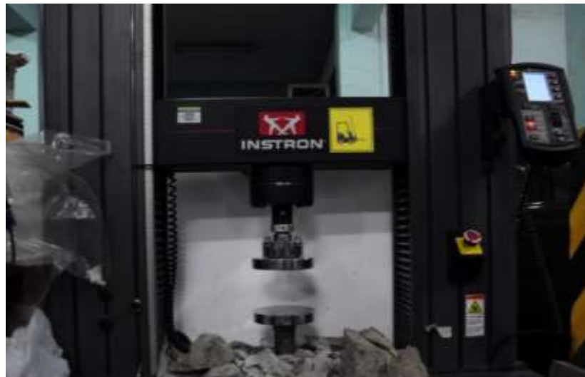
Figure 4. Instron 5982 floor model 100 kN capacity Universal Testing Machine with the control panel shown on the upper right.
