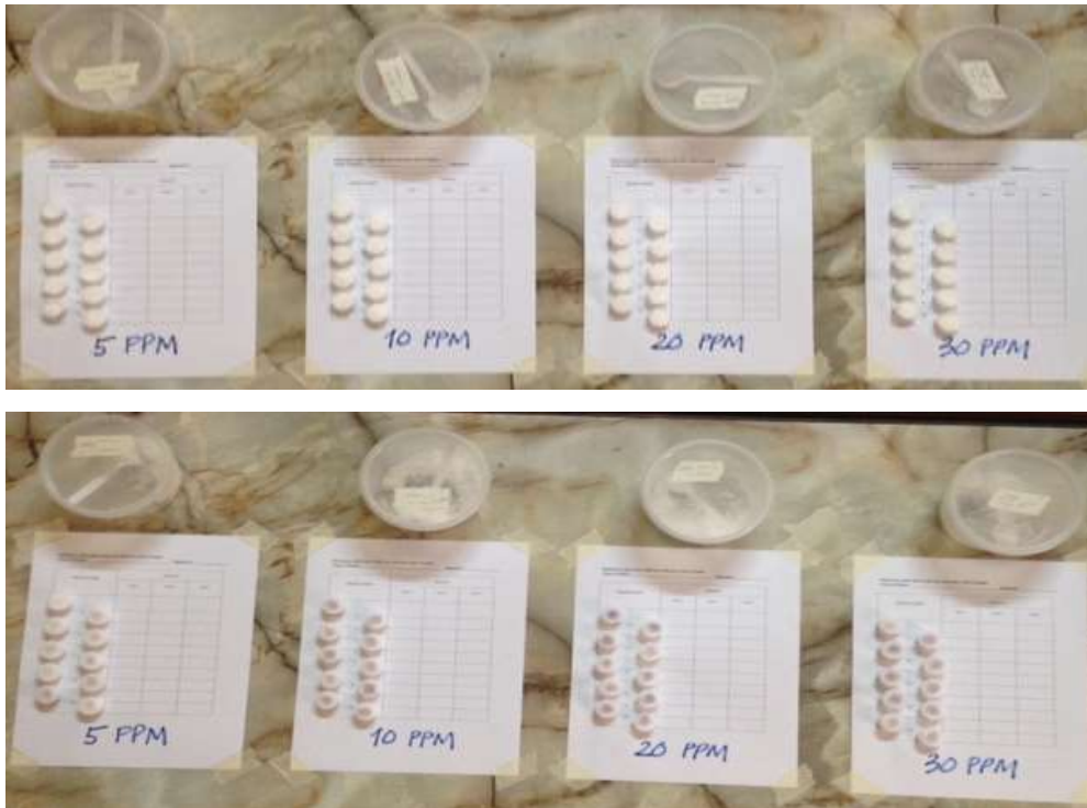
Figure 9. Prepared Samples for Attribute Gage R&R Study (above); Same Same Samples After Application of Test Solution (below)
