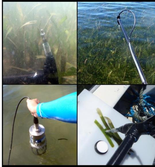
**Figure 4.** Fieldwork for spectral data measurement (Upper left: Measurement of underwater irradiance; *Upper right: Measurement of seagrass bed reflectance above water; Lower left: Water quality measurement using AAQ; Lower right: Reflectance measurement of seagrass samples.*)
