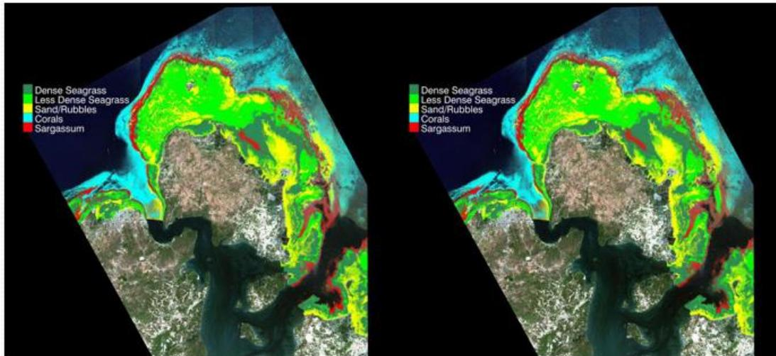
Figure 11. Classified Images of Stumpf’s Ratio Model using *Band Combination 1, 3, 4, 5 (left) and 2, 3, 4, 5 (right)*
