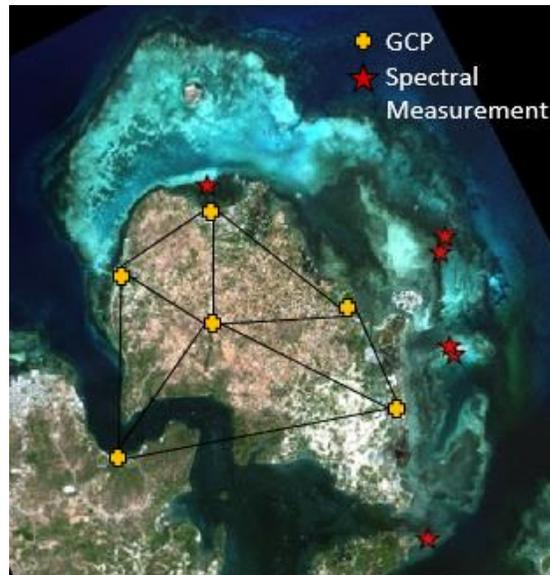
**Figure 3.** Ground control points (GCPs) indicated by yellow crosses and spectral data measurement sites indicated by red stars
