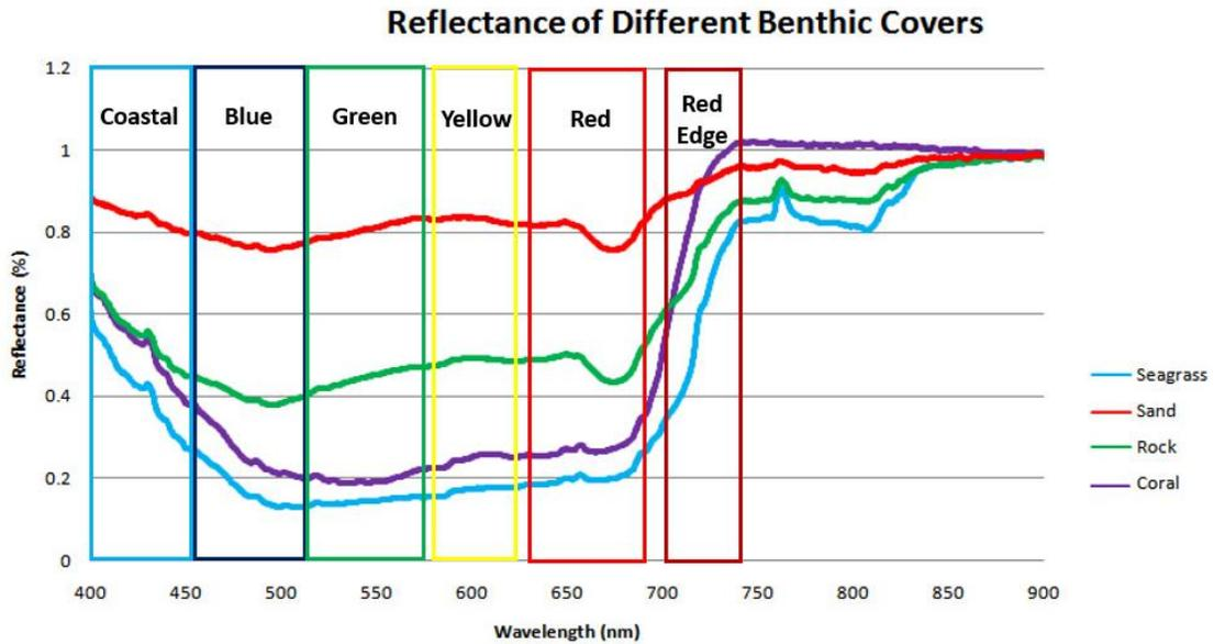
**Figure 9.** Comparison of underwater reflectance values of different benthic covers with the corresponding band ranges of WorldView-2
