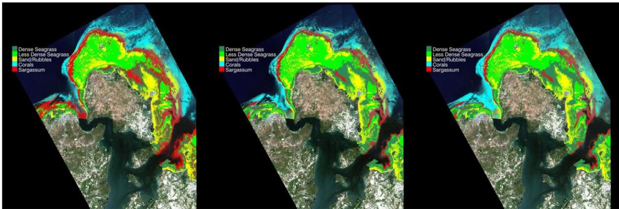
**Figure 10.** Maximum Likelihood Classified Images with Band Combination 1,3,4,5 (from left to right) using Lyzenga's Optical Model, Simple Radiative Transfer Model (SRTM) and Stumpf's Model
