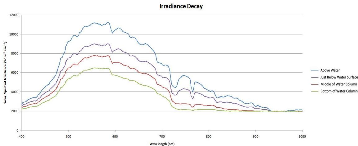
**Figure 8.** Irradiance decay as it goes deeper into the water column measured using a spectroradiometer
