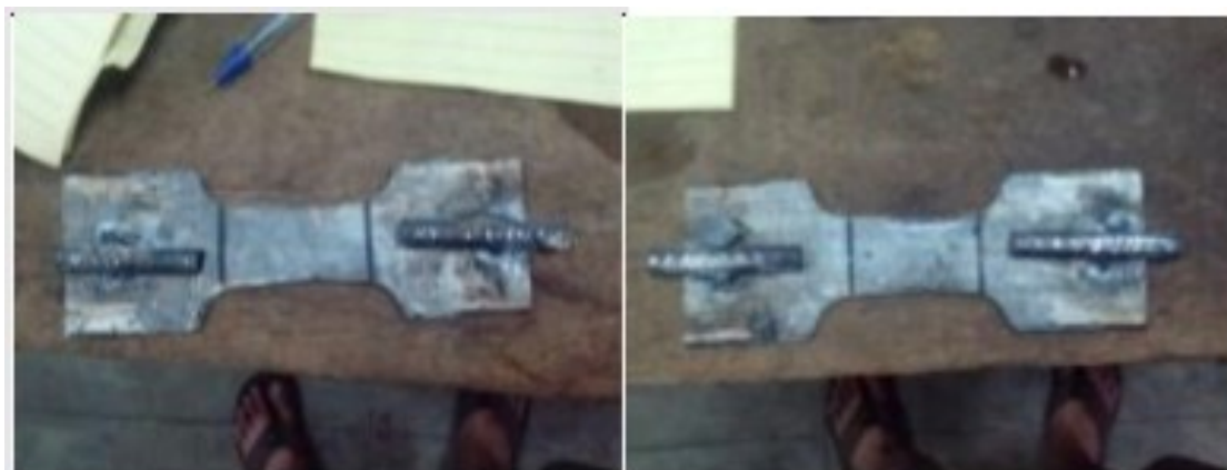
Figure 8. Flattened coupons that were cut from the sample, namely Sample 1 (left) and Sample 2 (right)
