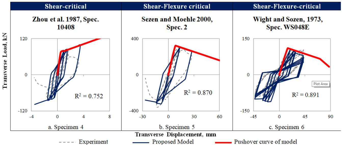
Figure 4. Cyclic loading of specimens 4 to 6.
