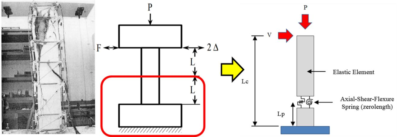
**Figure 1.** Cyclic loading of RC columns: (a) Actual column [19] (b) experimental setup (double cantilever) [20] (c) numerical model of proposed hinge.
