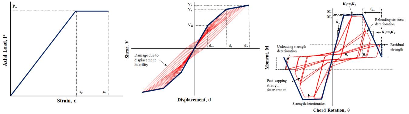
**Figure 2.** Hinge Parameters and Nonlinear Hysteresis model for (a) Axial (b) Shear and (c) Flexure.
