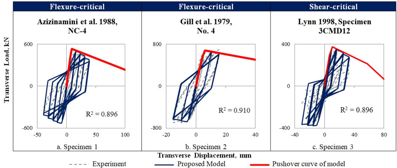
Figure 3. Cyclic loading of specimens 1 to 3.
