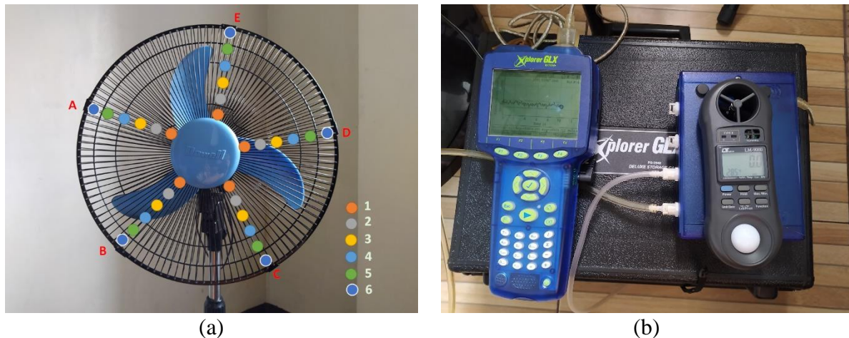
Figure 4: (a) Actual Fan (b) Pressure and Velocity Measurement Devices (Pasco Xplorer GLX)
