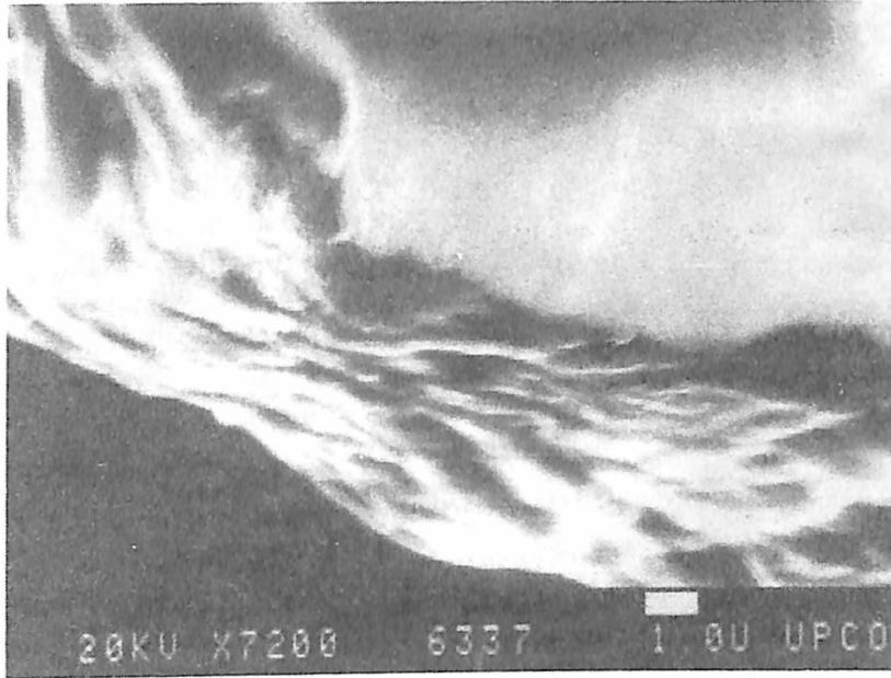
Figure 5. SEM photomicrograph of the cross-section of the polyester textile sample after soaking in HOAc-CaAc buffer solution. 20 kV, 7200 x mag.
