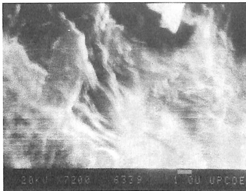
Figure 7. SEM photomicrograph of the cross-section of the polyester textile sample after soaking in \text{NaHCO}_3\text{-Na}_2\text{CO}_3 buffer solution. 20 kV, 7200 x mag.
