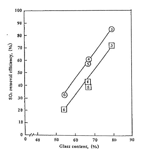
Figure 2. Correlation Between SO<sub>2</sub> Removal Efficiency and Glass Content Using Unsieved Fly Ash Samples
