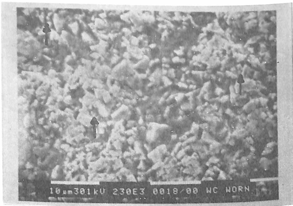
Figure 6. SEM of worn insert taken from the impact face of the percussive drill bit showing fragmented WC grains
