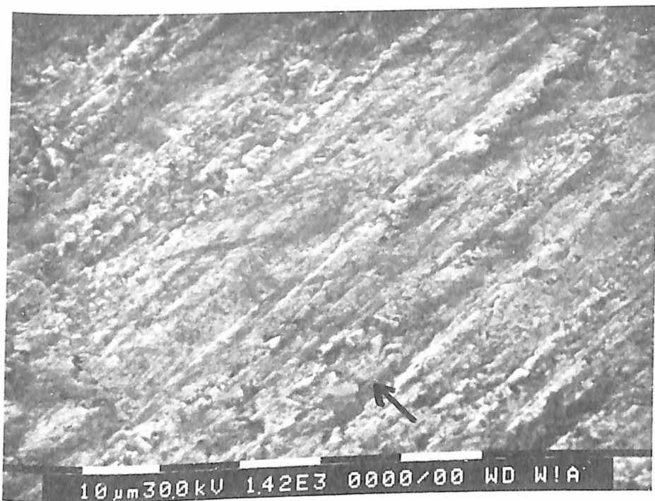
Figure 10. SEM micrograph showing partially cut WC-Co composite after abrasion with alumina abrasive.
