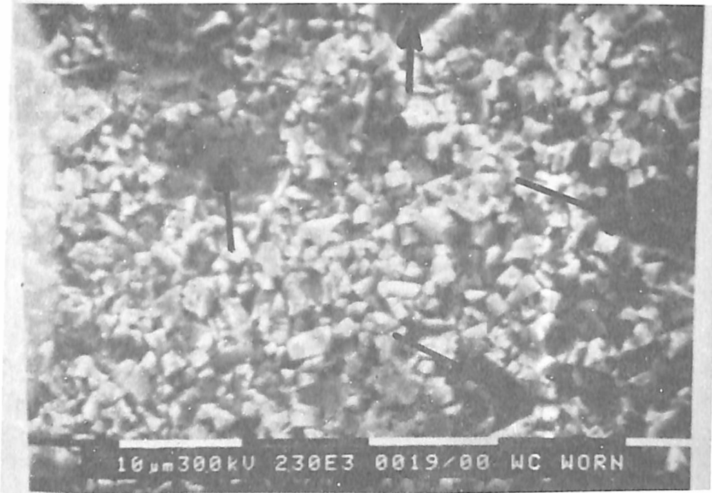
Figure 7. Wear scar of the insert showing gross pull out of WC grains due to impact fatigue
