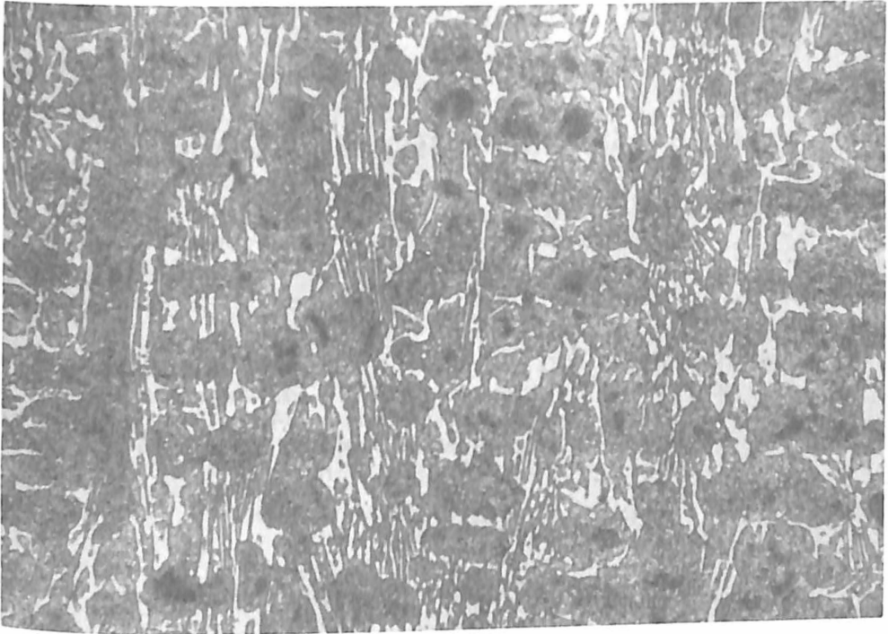
Figure 9. Shell microstructure of a typical high chromium hot mill roll
