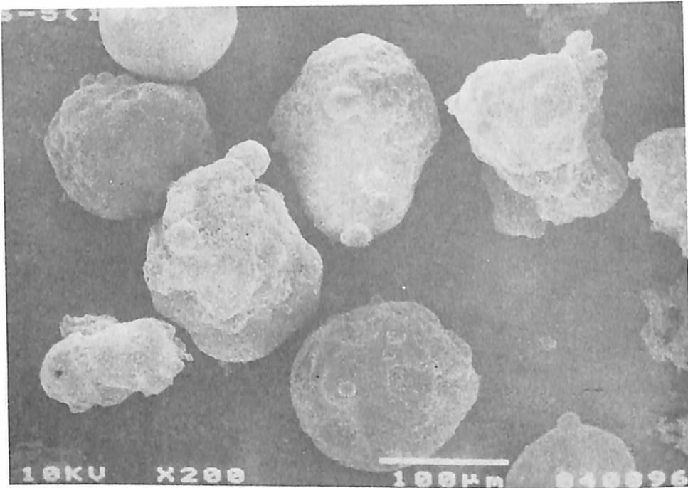
**Figure 9a.** Morphological Structure of 1996 Coal Ash Sample
