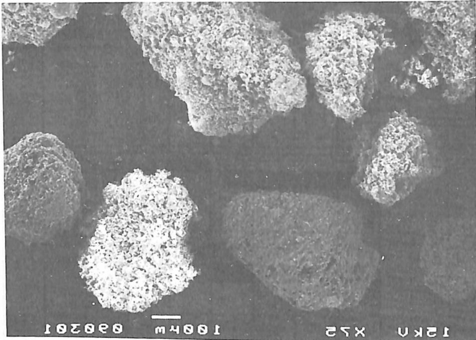
Figure 8a. Morphological Structure of 1993 Coal Ash Sample
