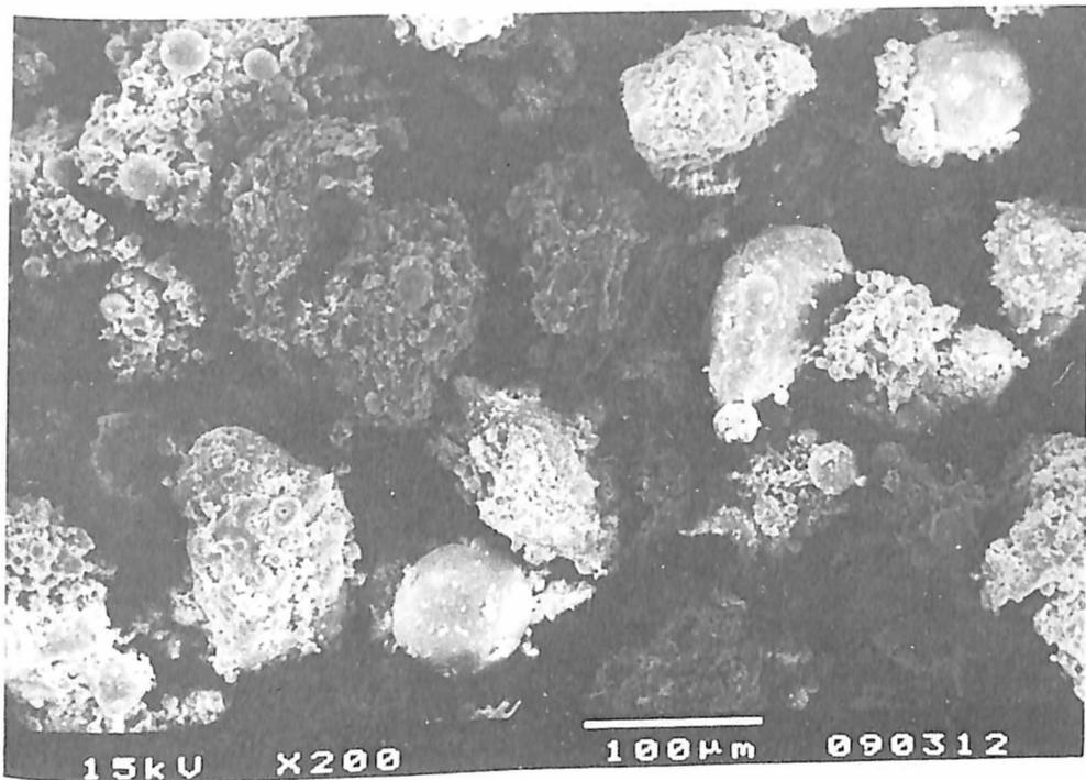
**Figure 8d.** Morphological Structure of 1993 Coal Ash Sample
