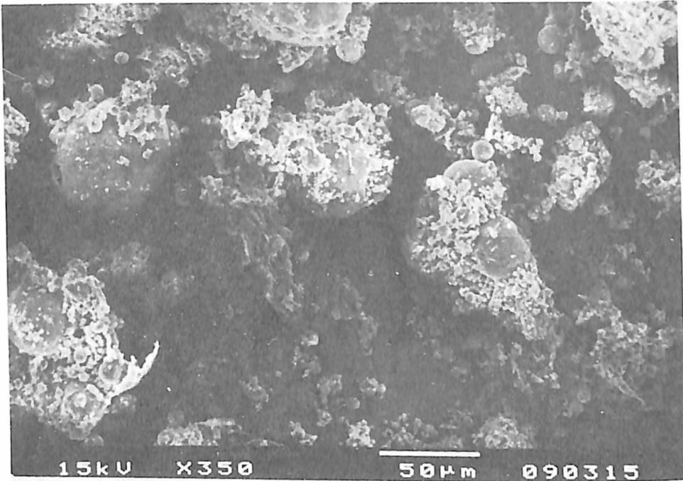
Figure 8e. Morphological Structure of 1993 Coal Ash Sample
