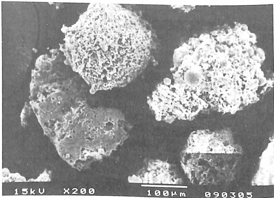
Figure 8b. Morphological Structure of 1993 Coal Ash Sample
