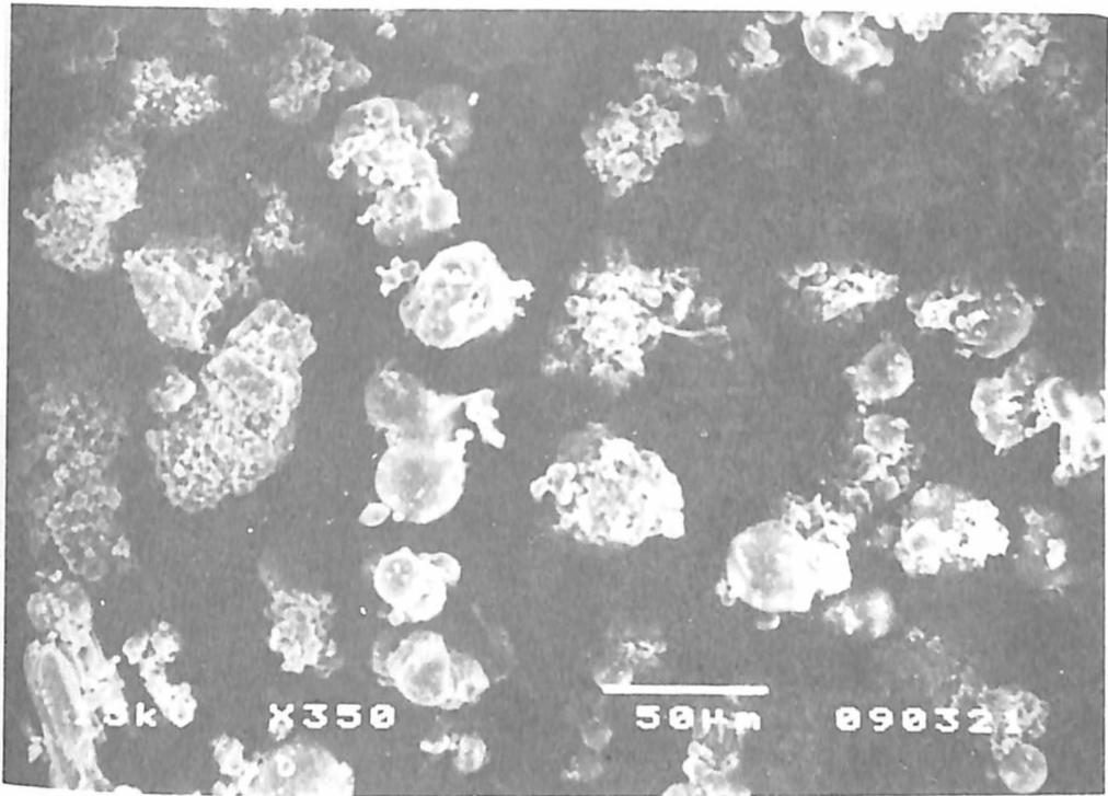
Figure 8g. Morphological Structure of 1993 Coal Ash Sample
