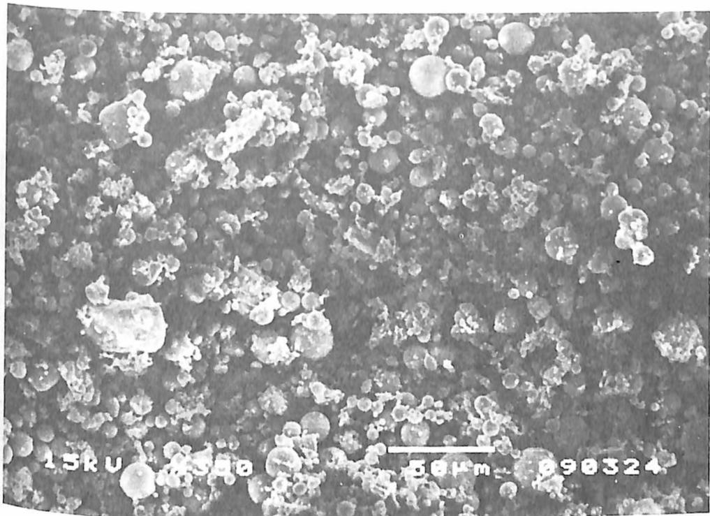
Figure 8h. Morphological Structure of 1993 Coal Ash Sample
