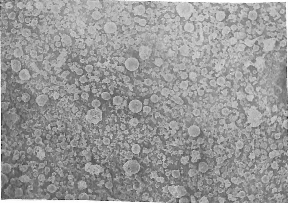
**Figure 9f.** Morphological Structure of 1996 Coal Ash Sample
