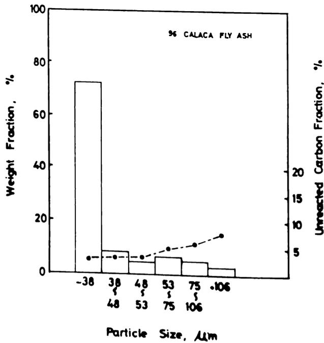
Figure 3. Weight Fraction vs. Unreacted Carbon for each Particle Size (1996 Coal Ash Samples)
