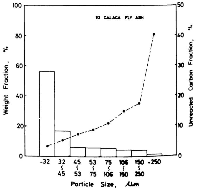
Figure 2. Weight Fraction vs. Unreacted Carbon for each Particle Size (1993 Coal Ash Samples)
