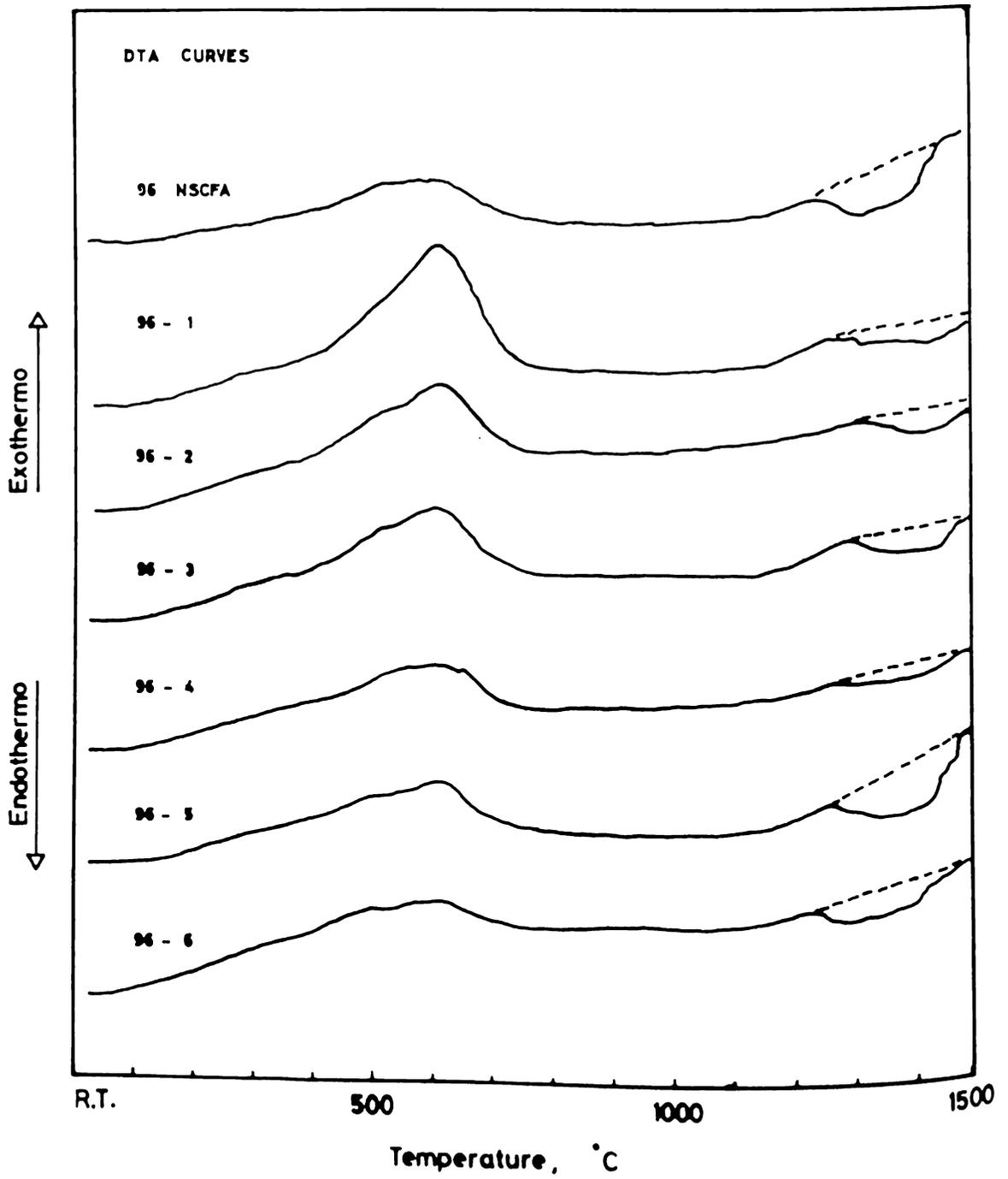
Figure 11. Thermal Analysis of each Particle Size of the 1996 Coal Ash Samples
