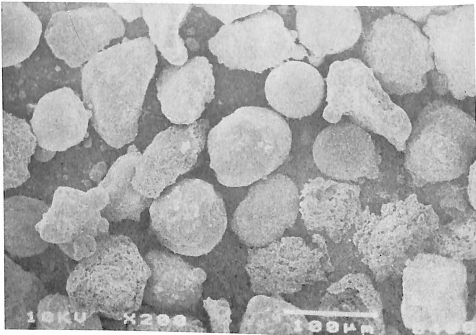
**Figure 9b.** Morphological Structure of 1996 Coal Ash Sample
