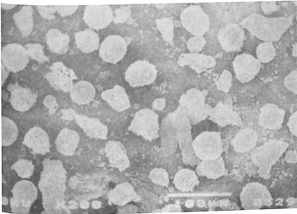
**Figure 9d.** Morphological Structure of 1996 Coal Ash Sample
