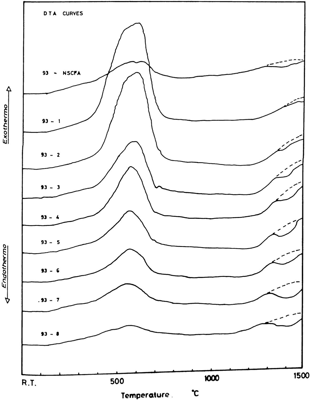
Figure 10. Thermal Analysis of each Particle Size of the 1993 Coal Ash Samples
