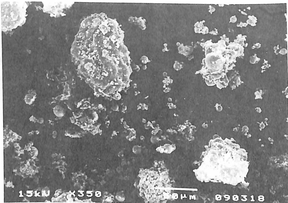
Figure 8f. Morphological Structure of 1993 Coal Ash Sample
