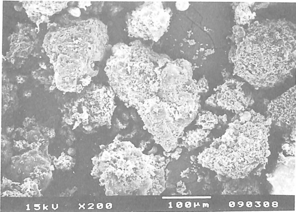
**Figure 8c.** Morphological Structure of 1993 Coal Ash Sample
