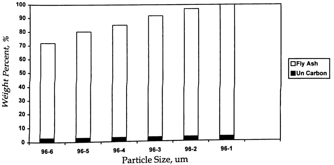
Figure 5. Cumulative Weight Fraction vs. Unreacted Carbon for each Particle Size (1996 Coal Ash Samples)
