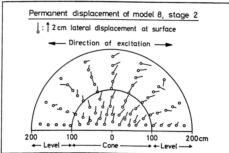
Figure 12: Permanent displacement of Model 8 test at PWRI (after Sasaki et al., 1991)
