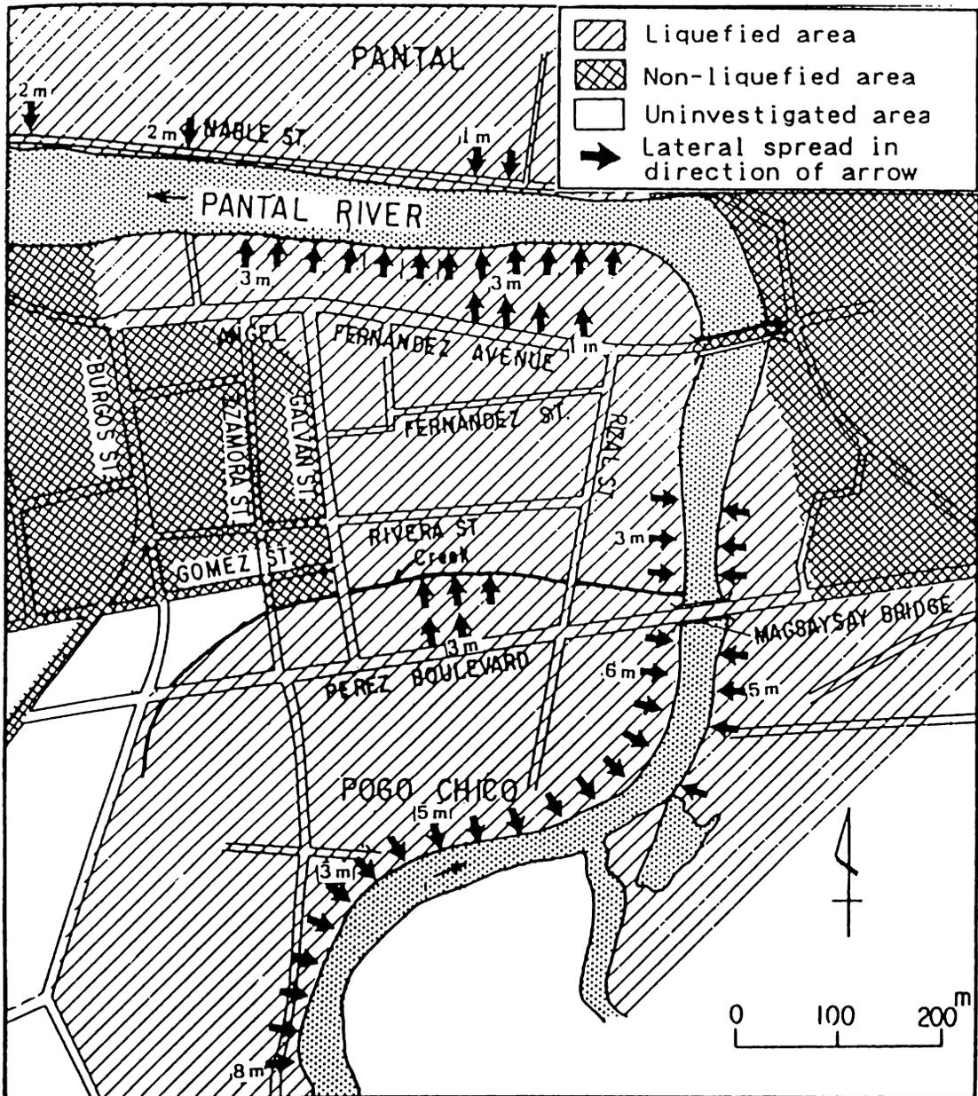
Figure 5: Approximate extent of liquefaction in Dagupan City (after Wakamatsu et al., 1991)
