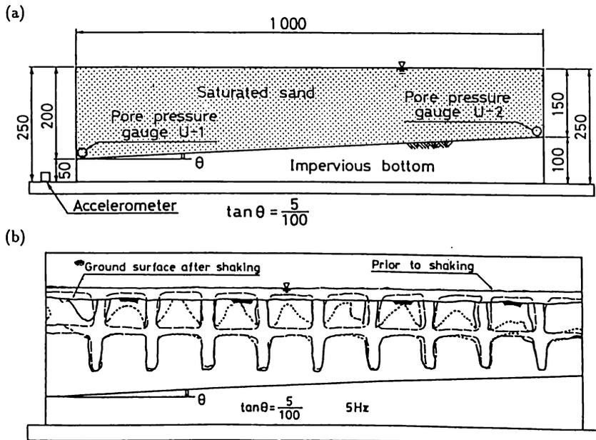
Figure 10: Model ground with flat surface and inclined (a) experimental set-up; (b) ground deformation
