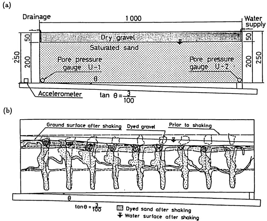
Figure 9: Model ground with inclined water table: (a) experimental set-up; (b) ground deformation
