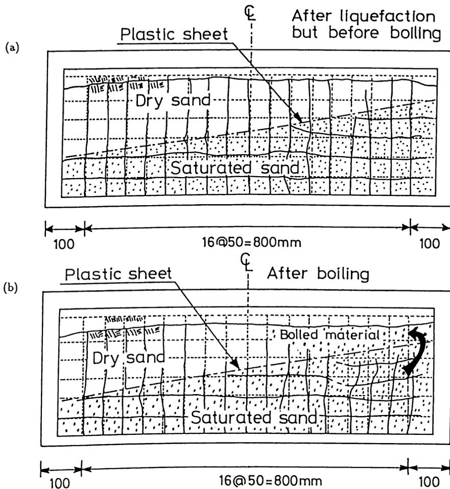
Figure 8: Configuration of model ground in which dry layer was underlain by water saturated one with inclined surface: (a) after liquefaction but before boiling; (b) after boiling
