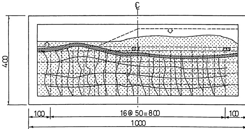
Figure 7: Deformation of model ground with small embankment on the surface
