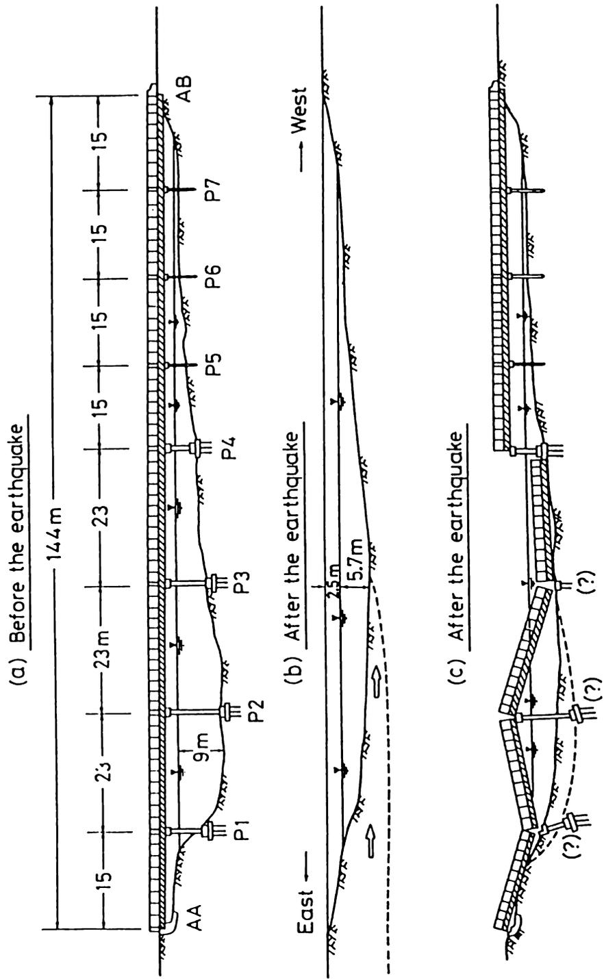
Figure 6: Sketch of Magsaysay Bridge before and after the earthquake (after Ishihara et al., 1993)
