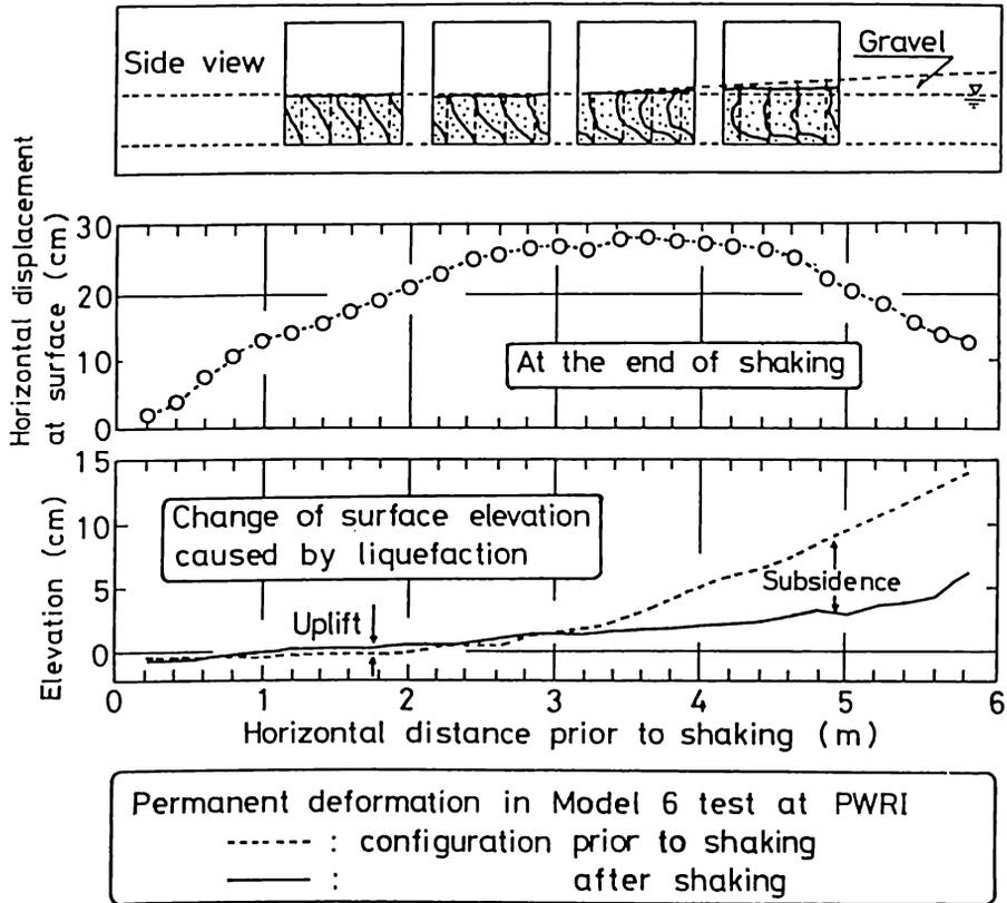
Figure 11: Permanent displacement of Model 6 test at PWRI (after Sasaki et al., 1991)
