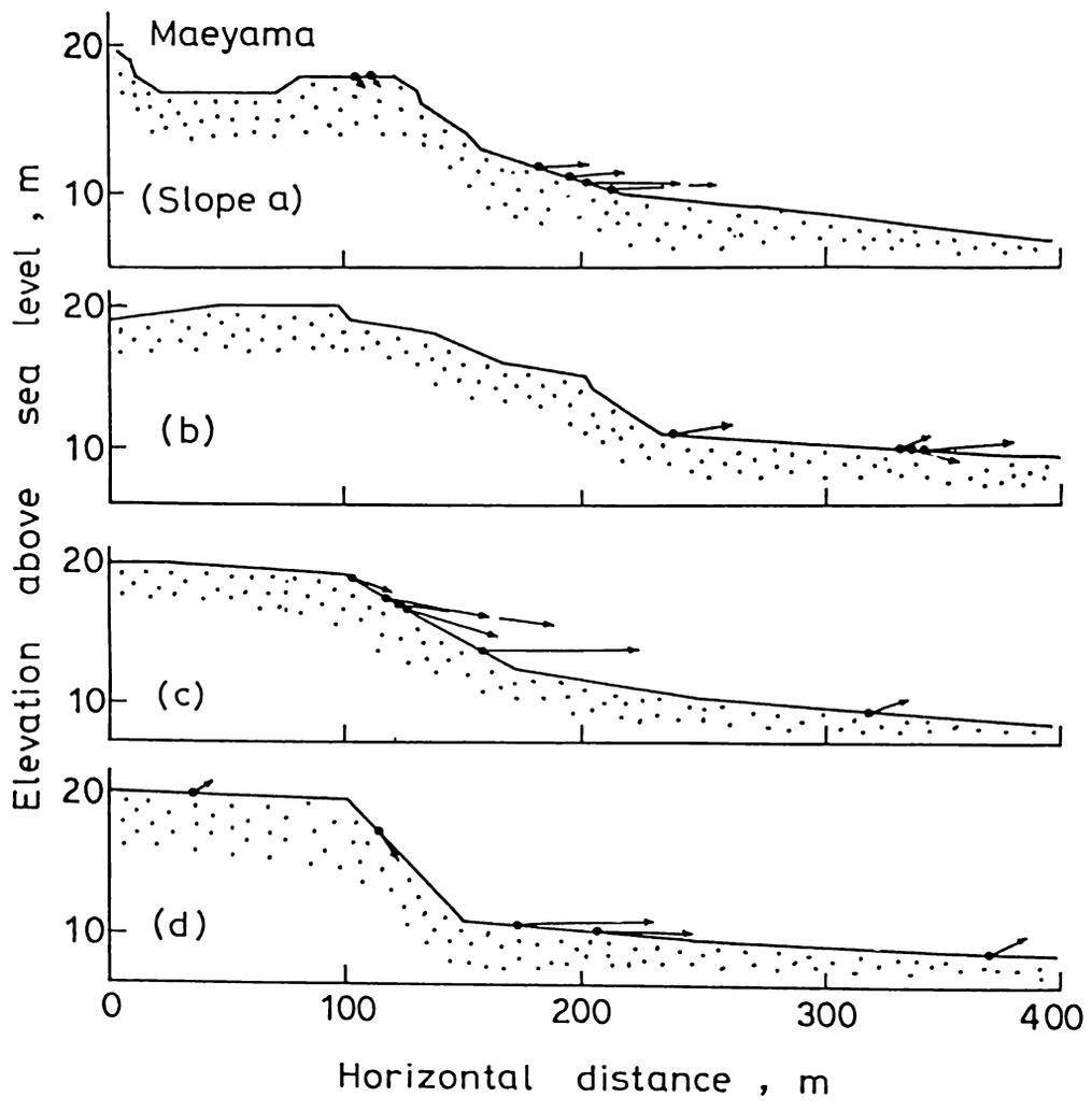
Figure 4: Ground movement in cross sections of Mae Hill slope
