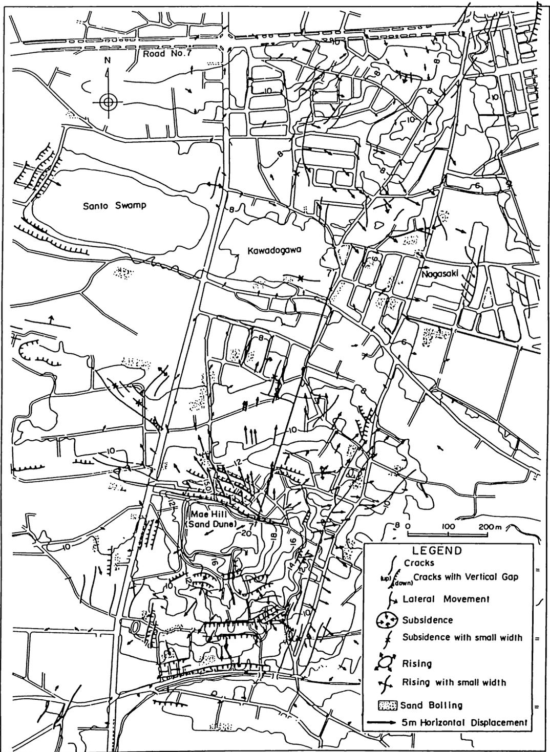
Figure 3: Permanent horizontal ground displacements in Noshiro City (after Hamada et al., 1986)
