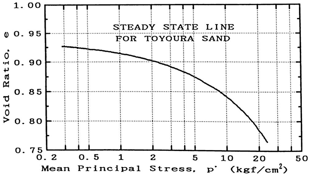
Figure 14: Relation between effective stress and void ratio at steady state for Toyoura sand (after Verdugo et al., 1991)
