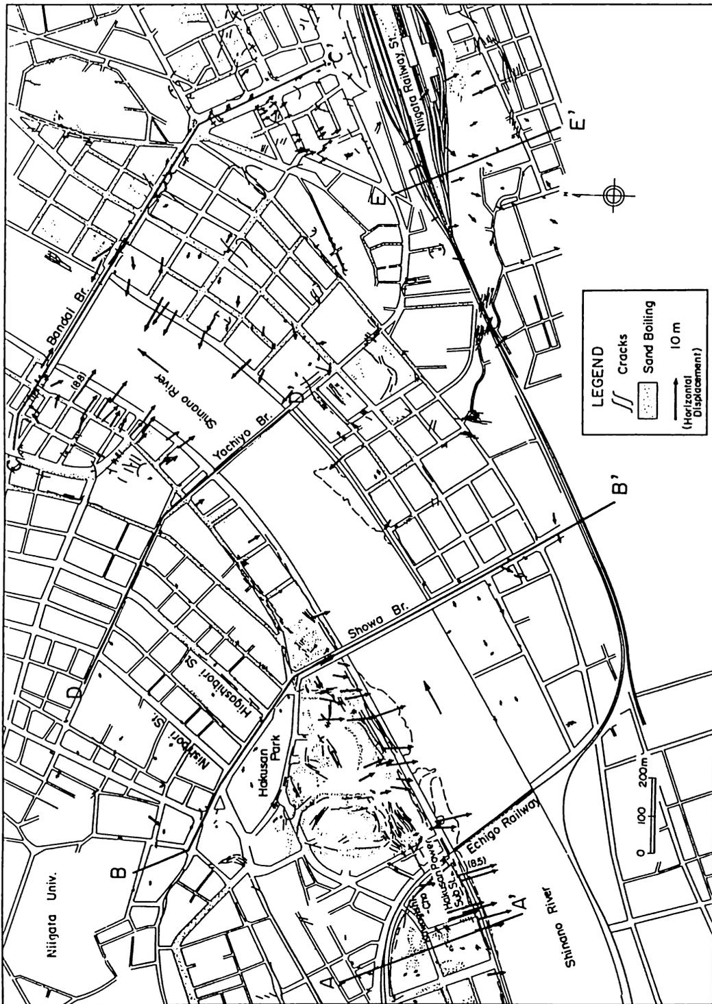
Figure 1: Permanent horizontal ground displacements in Niigata City (after Hamada et al., 1986)
