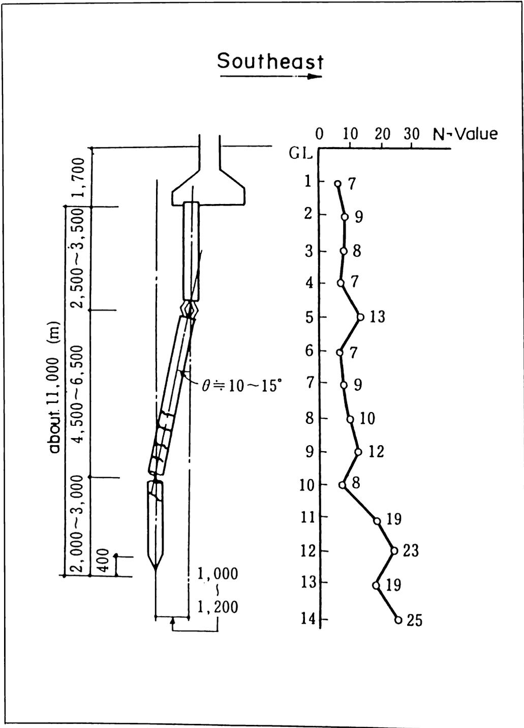
Figure 2: Broken pile in Niigata City (after Kawamura et al., 1985)
