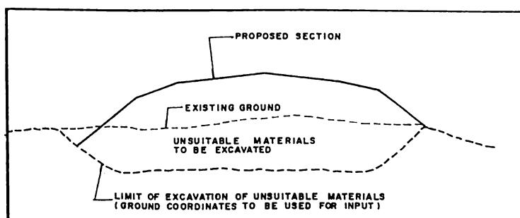
Figure 3a. TYPE 1 - TREATMENT (EXCAVATION OF UNSUITABLE MATERIALS)
