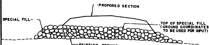
Figure 3b. TYPE 2 - TREATMENT (USE OF SPECIAL FILL)
