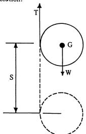
The free body diagram of the cylinder is shown at the left. The traditional work energy equation (Eq. 7) yields
