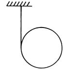
A flexible cord is wrapped around a cylinder of weight W. Find
