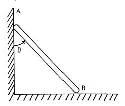
The homegeneous bar AB of length  $\ell$  and weight W is released from rest when  $\Theta=0$ . Neglecting friction, find the angular velocity of the rod and the reactions at A and B in terms of  $\Theta$ .
