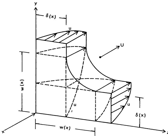
Figure 2. The  $x$ -component velocity profile,  $u(x,y,z)$
