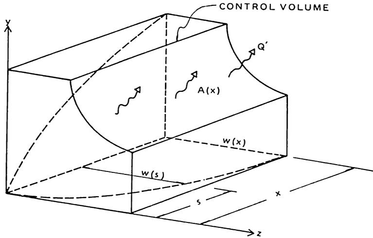
Figure 3. The control volume for the integral formulation
