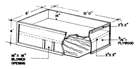
Fig. 4 . DRYING BIN DETAILS
