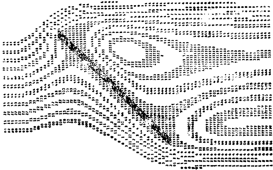
Fig. A.4(b) Laminar flow past an inclined plate after command MASK.
