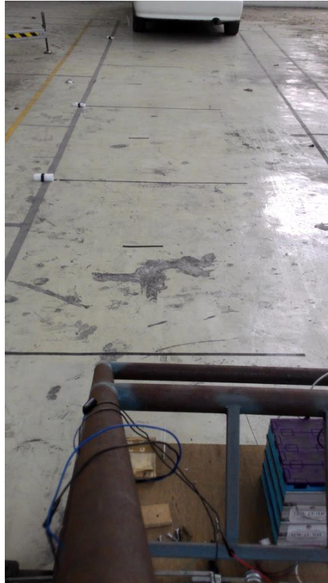
Figure 9. A snippet from the recordings of an indoor test showing the road markings in the indoor test
