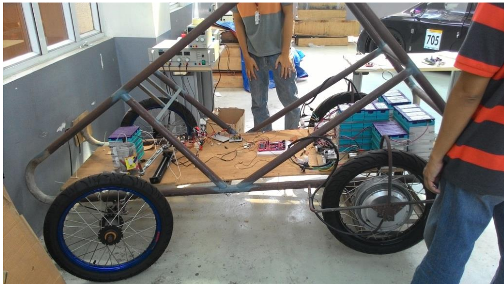
Figure 7. Fabricated EV's frame with the essential car parts only: chassis, in-tire motors, battery packs, and controller.
