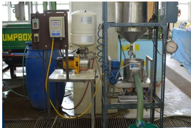
Figure 2. The L40 Falcon Gravity Concentrator used for concentration tests
