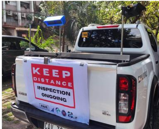
Figure 2. Camera mounted on a vehicle.
